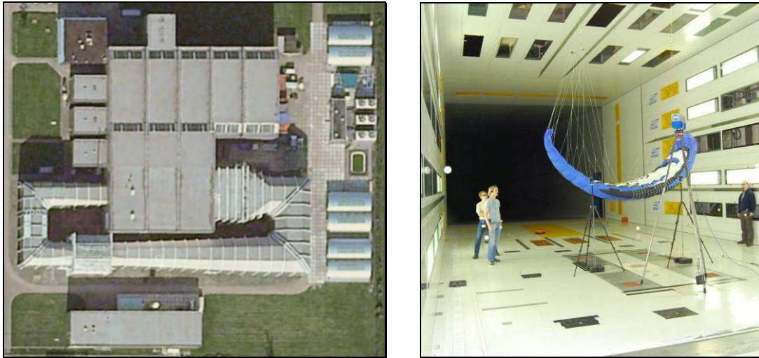
Figure 5.4: Top view of the LLF windtunnel [Source: Google Earth] and view of the 8 x 6m test section with the kite.
