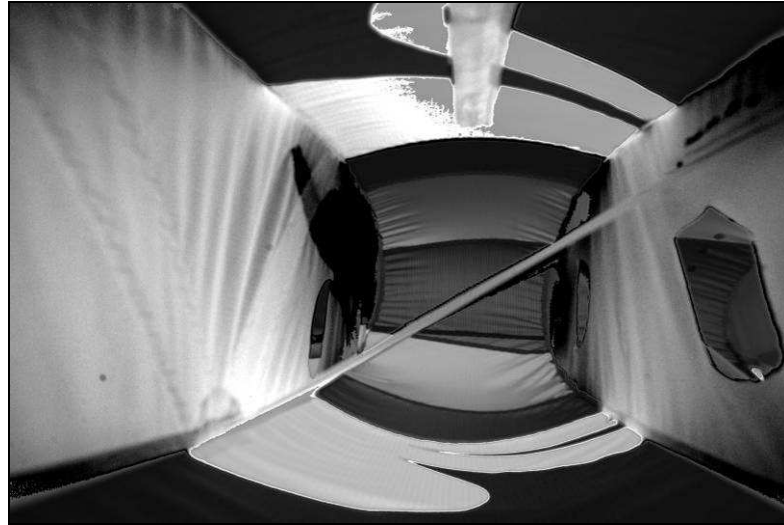
Figure 6.19: Wrinkles from the top and bottom surface continue in the ribs.
