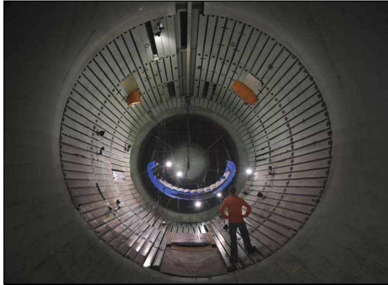
Figure 5.12: The kite suspended in the Böenwindkanal. [Source: Max Dereta]
