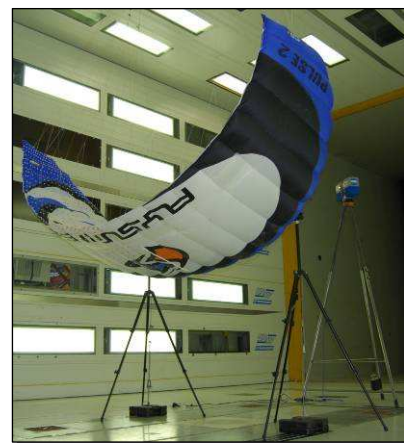
Figure 5.15: The kite in the LLF tunnel with the laser scanner on a tripod.
