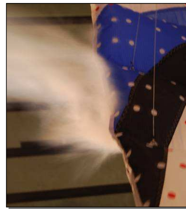
Figure 6.12: Smoke accumulates at the thick trailing edge.
