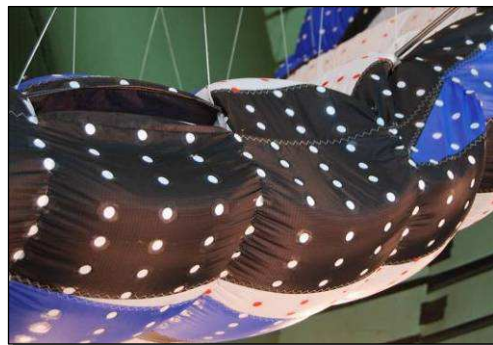
Figure 5.18: Dents appear in the leading edge when the angle of attack becomes small.
