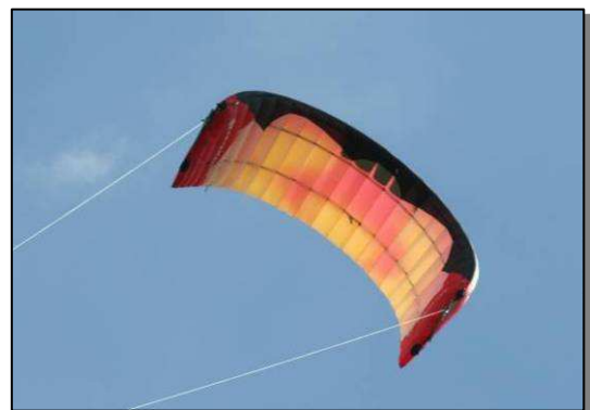
Figure 2.2: The C-shaped ram-air kite of the Laddermill.
