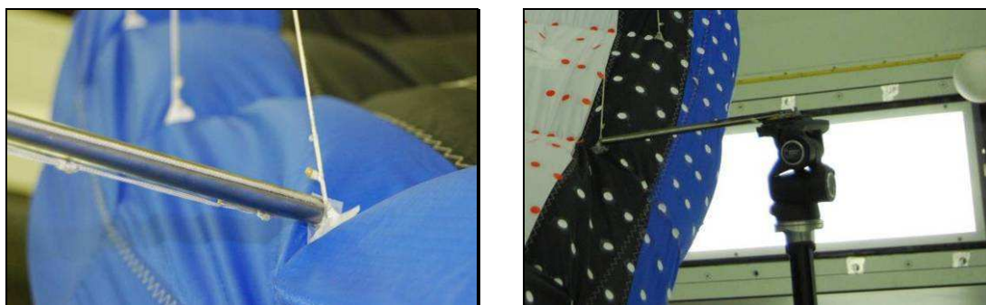
Figure 5.10: The fixation tripods lashed to the line attachment points.
