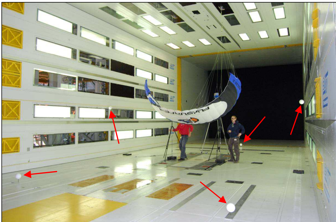
Figure B.2: The registration spheres placed in the windtunnel.
