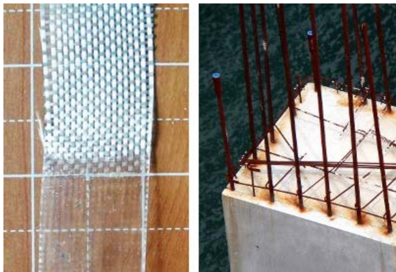
Figure 2.4: Glass fiber reinforcement partially covered by resin matrix (left) and steel reinforcement partially covered by concrete matrix (right). [GS Consulting, Emporis]
