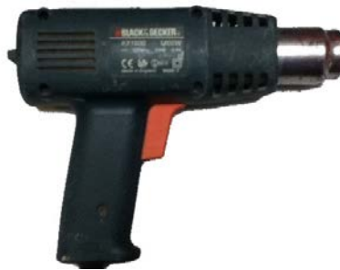
Figure 8.6: Black & Decker 1400 watt heat gun, which was used to locally heat the elastic foil samples.
