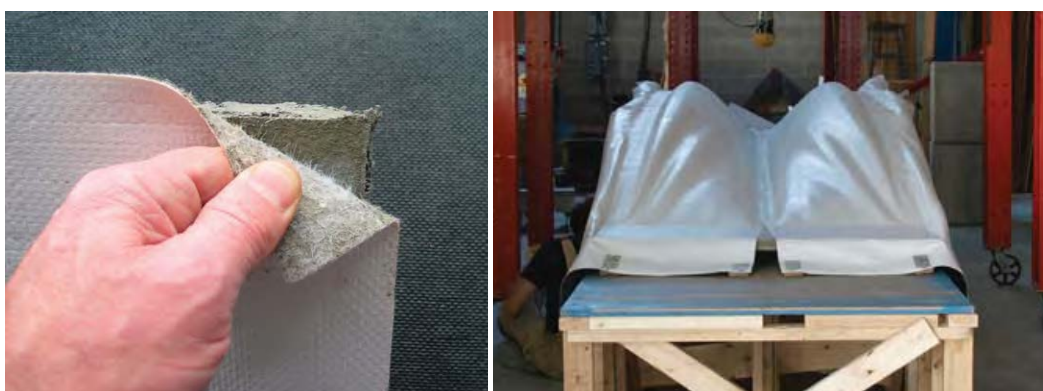
Figure 3.6: Fabrene "Development Product W756" with fuzzy side bonded to concrete and mold showing buckled fabric "musculature". [West]
