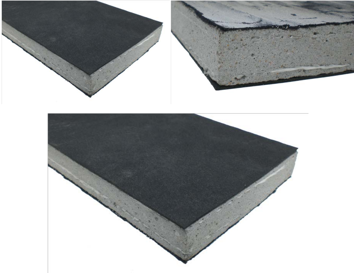
Figure 5.16: Photos of the physical prototype of the material showing reinforcement, concrete matrix, black elastic layer, and grey-black cloth layer, measuring approximately 20mm thick, 100mm wide, and 200mm long.
