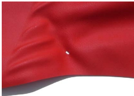
Figure 8.8: Hole in shear deformed elastic film in elevated temperature conditions.
