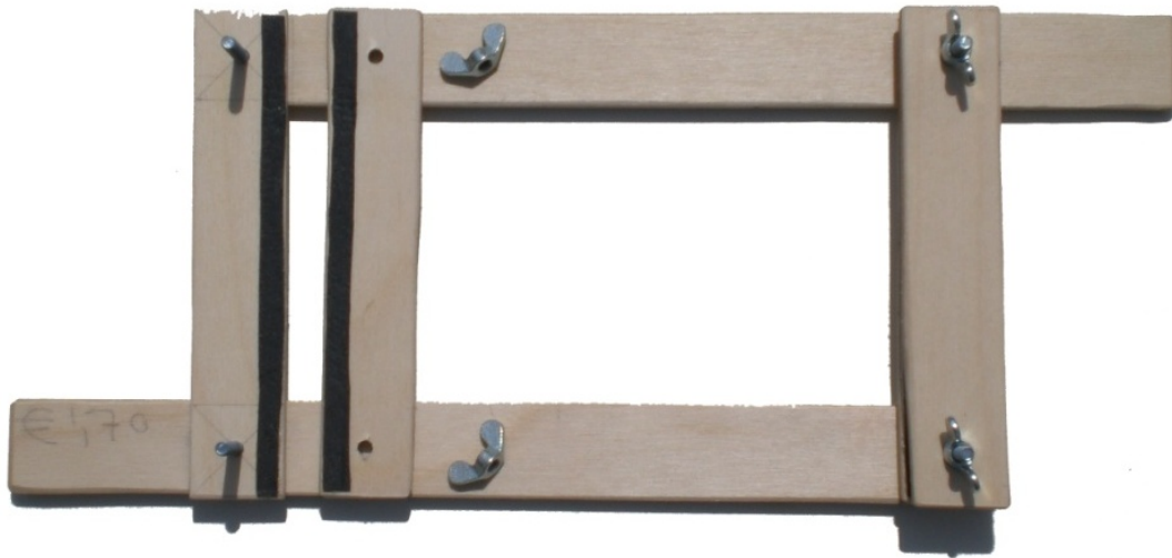
Figure 8.1: Shear testing device with one clamp disassembled, showing black rubber grip pads.
