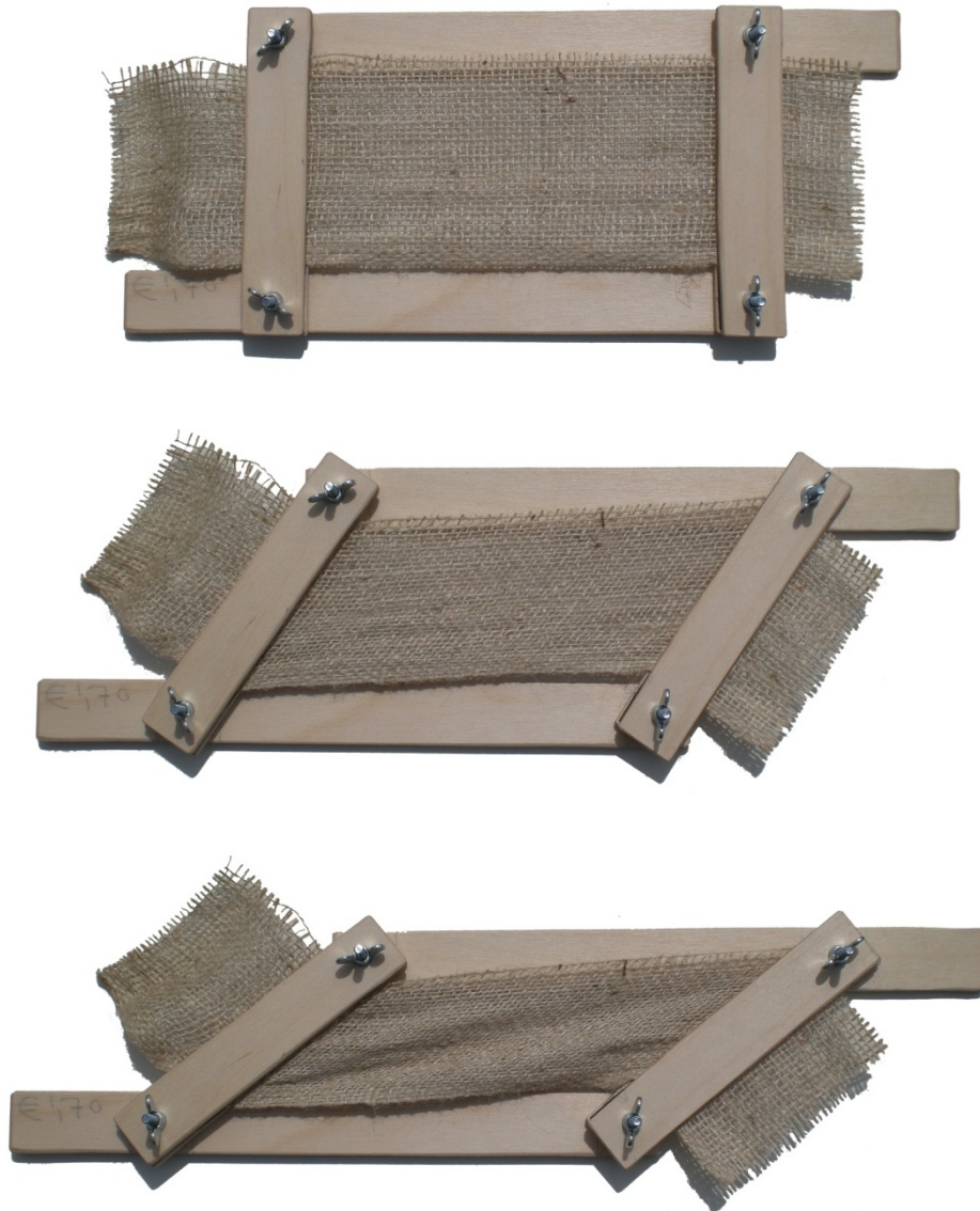
Figure 8.3: Deformation of a woven burlap sample from 90° down to 40°, showing slight buckling at 40°.
