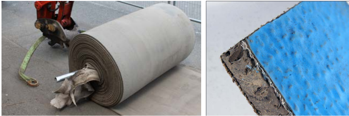
Figure 0.3: Bulk roll of Concrete Canvas and close-up. [Concrete Canvas]
