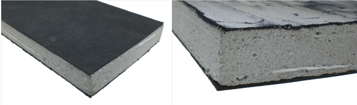
Figure 0.5: Photos of the physical prototype of the material showing reinforcement, concrete matrix, black elastic layer, and grey-black cloth layer, measuring approximately 20mm thick, 100mm wide, and 200mm long.
