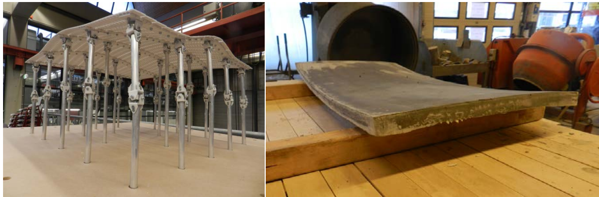
Figure 3.7: Controllable mold and double-curved concrete panel with woven glass reinforcement. [Eigenraam, Kok]
