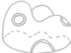
ISOTROPIC CONSTANT THICKNESS HOLES + STIFFENERS
