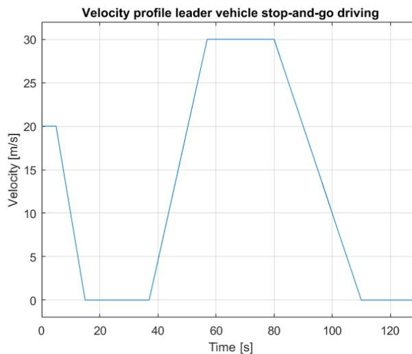
**Figure 5-2:** Velocity profile leader vehicle for stop-and-go scenario
