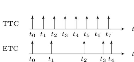
**Figure 1-2:** Time Triggered Control (TTC) versus Event Triggered Control (ETC) with respect to actuator update instants. [3]
