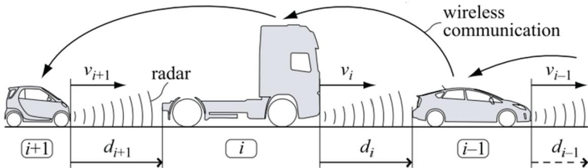
**Figure 2-1:** A vehicle platoon consisting of non-identical vehicles. All vehicles are equipped with a speed sensor measuring the vehicle speed  $v_i$ , a radar measuring the intervehicle distance  $d_i$ , sensor to measure the vehicle's acceleration, and hardware to communicate with a following vehicle. [8]
