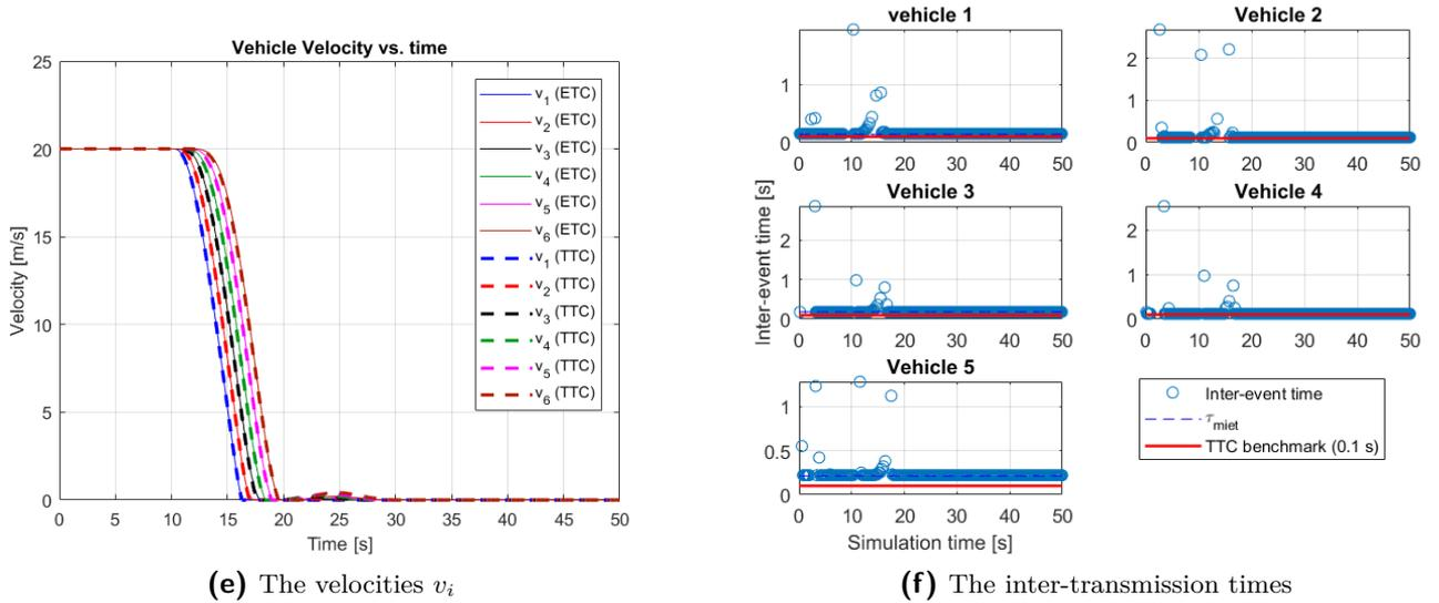
**Figure 5-3:** The simulation results for emergency braking
