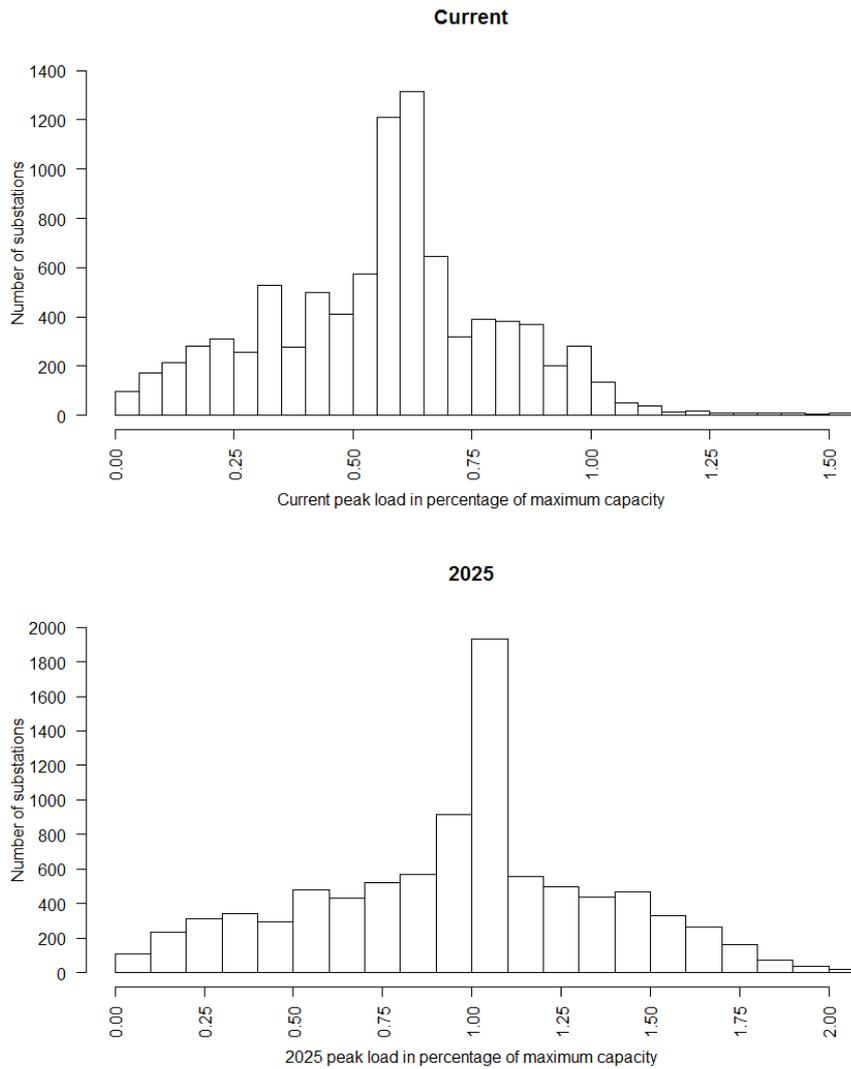
Figure 3.15: Histograms of current and 2025 peak load for all substations controlled by Stedin
