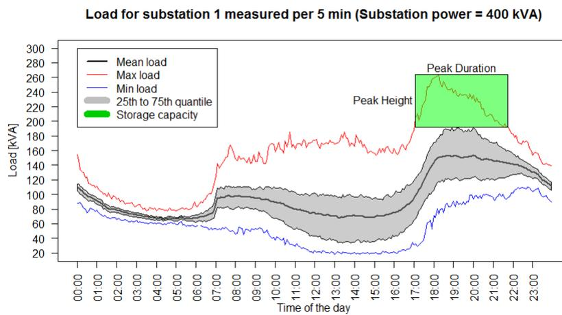
Figure 3.6: Load characteristics for all days of substation 1 (167 residential connections) with indication for the capacity of the storage
