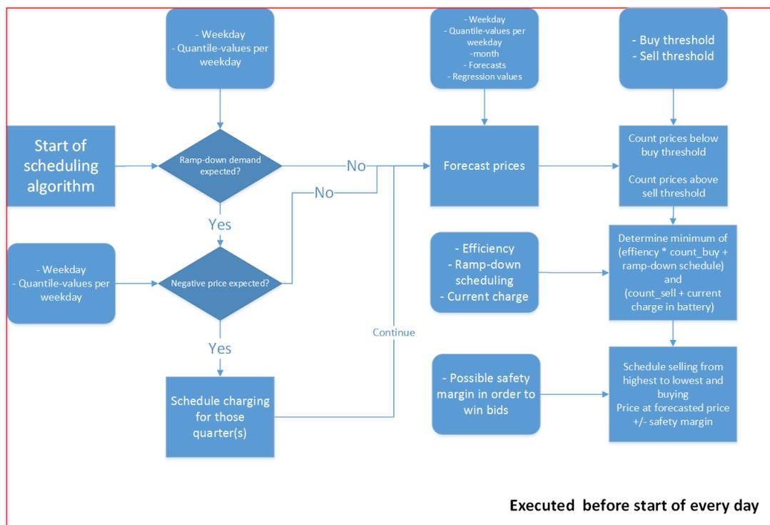
Figure 5.1: Conceptual scheme for the scheduling element of the trading algorithm
