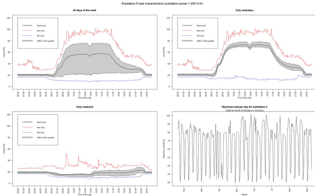
Figure 3.13: Load characteristics for substation 5 (15 non-residential and 1 residential connections) measured per 5 min for 01-01-2016 - 01-10-2016
