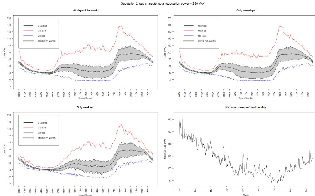
Figure 3.7: Load characteristics for substation 2 (158 residential connections, 1 non-residential) for 01-01-2016 till 01-10-2016
