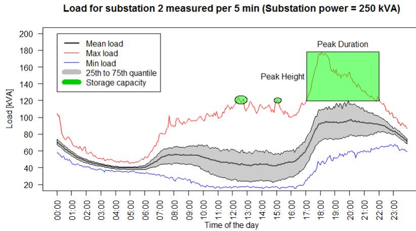
Figure 3.8: Load characteristics for all days of substation 2 (158 residential connections, 1 non-residential) with indication for the capacity of the storage
