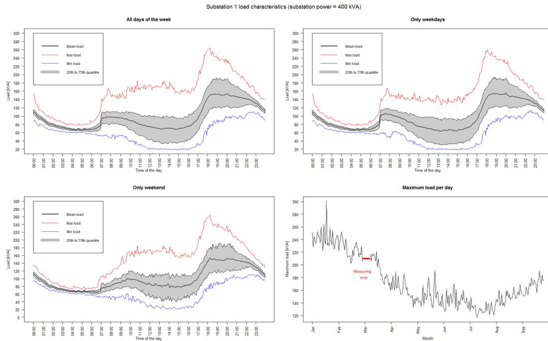
Figure 3.5: Corrected load characteristics of substation 1 (167 residential connections) for 01-01-2016 till 01-10-2016
