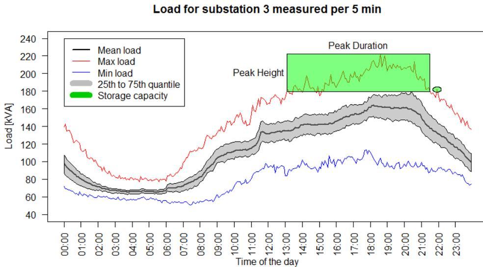
Figure 3.10: Load characteristics for all days of substation 3 (66 residential connections, 32 non-residential) with indication for the capacity of the storage
