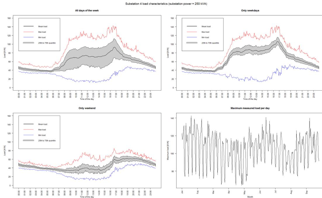
Figure 3.11: Load characteristics for substation 4 (11 residential and 32 non-residential connections) measured per 5 min for 01-01-2016 till 01-10-2016
