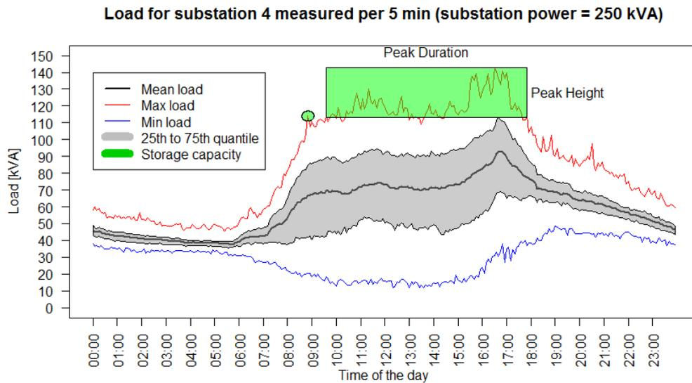
Figure 3.12: Load characteristics for all days of substation 4 (11 residential and 32 non-residential connections) with indication for the capacity of the storage
