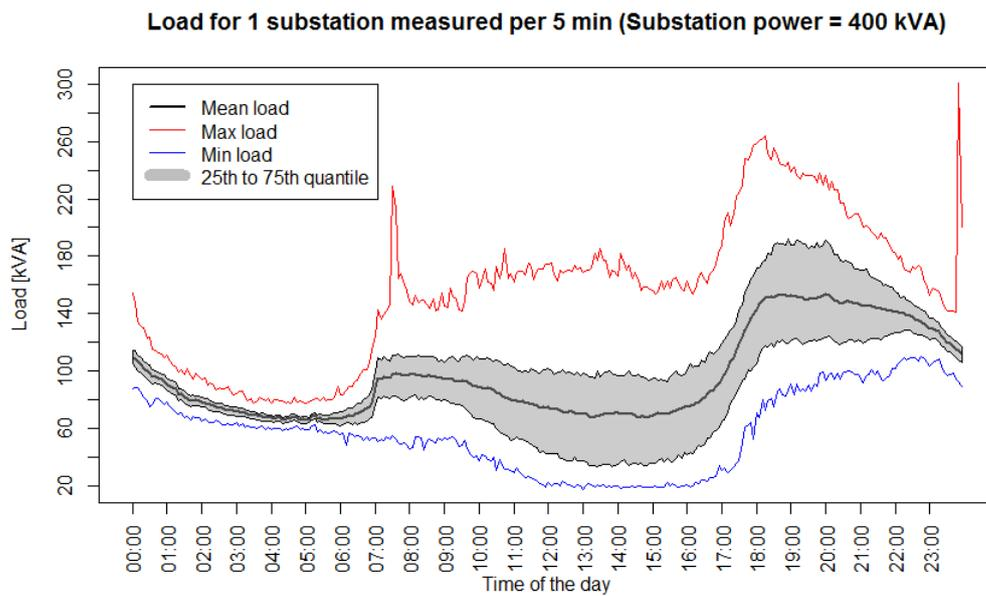
Figure 3.4: Load characteristics of substation 1 (167 residential connections) for 01-01-2016 till 01-10-2016
