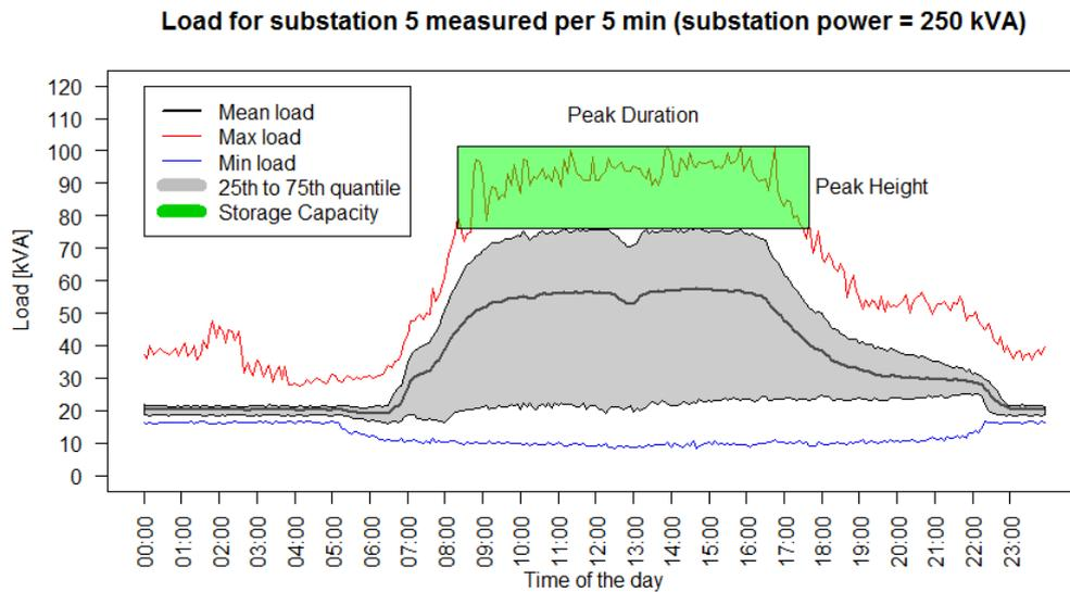
Figure 3.14: Load characteristics for all days of substation 5 (1 residential and 15 non-residential connections) with indication for the capacity of the storage
