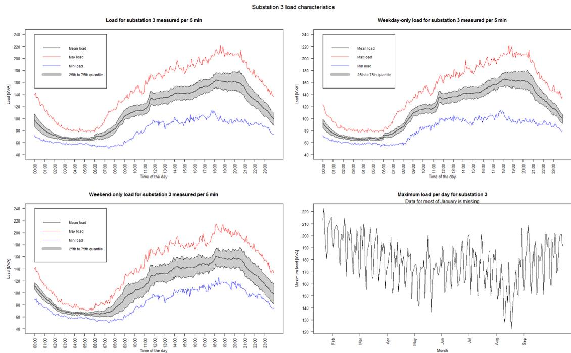
Figure 3.9: Load characteristics for substation 3 (66 residential and 32 non-residential connections) measured per 5 min for 01-01-2016 till 01-10-2016
