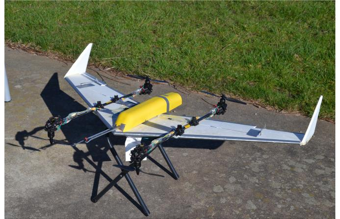
**Figure 1:** Dual-axis tilt-rotor quad-plane developed by Mancinelli et al. [2]. Photo courtesy of Nico Voß.
