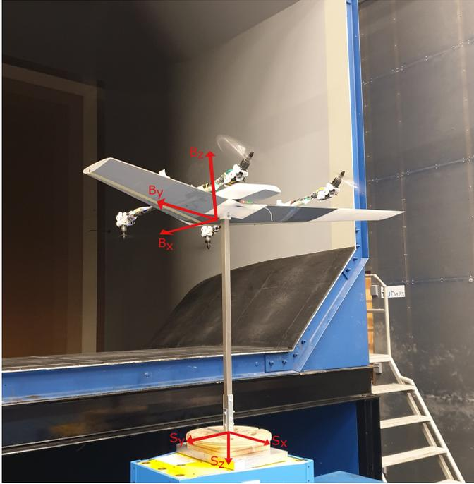
**Figure 5:** Wind tunnel experiment setup of the quad-plane, with sensor and body frames shown. Note that the drone is mounted upside down.
