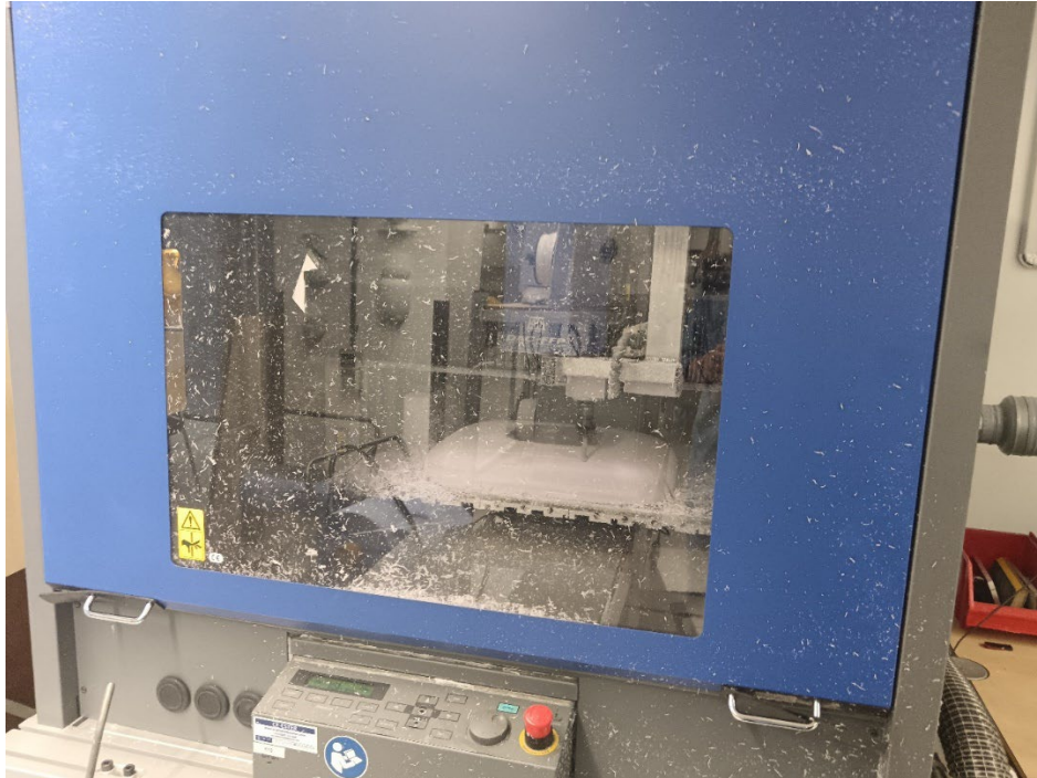
Figure 81: The manufacturing process - Mold for the back of the model being milled out of foam using the CAD model.
