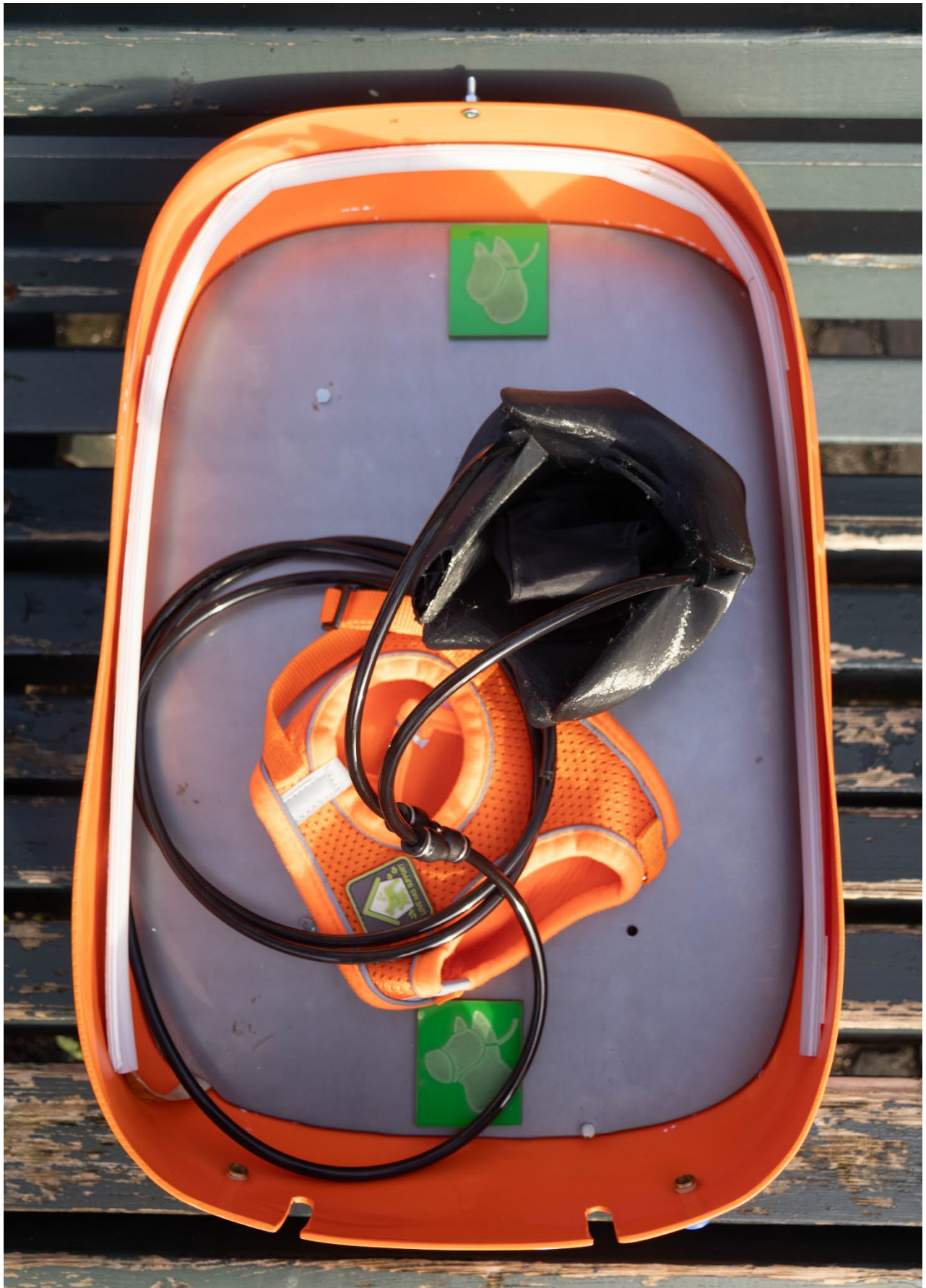
Figure 100: The device in its final stages of the design during the testing phase in public (see Chapter 7 – Final Tests and Redesign). The engraved plastic plaques attached to the metal sheet and the cat harness and the dog mask attached to the metal plate by magnets.
