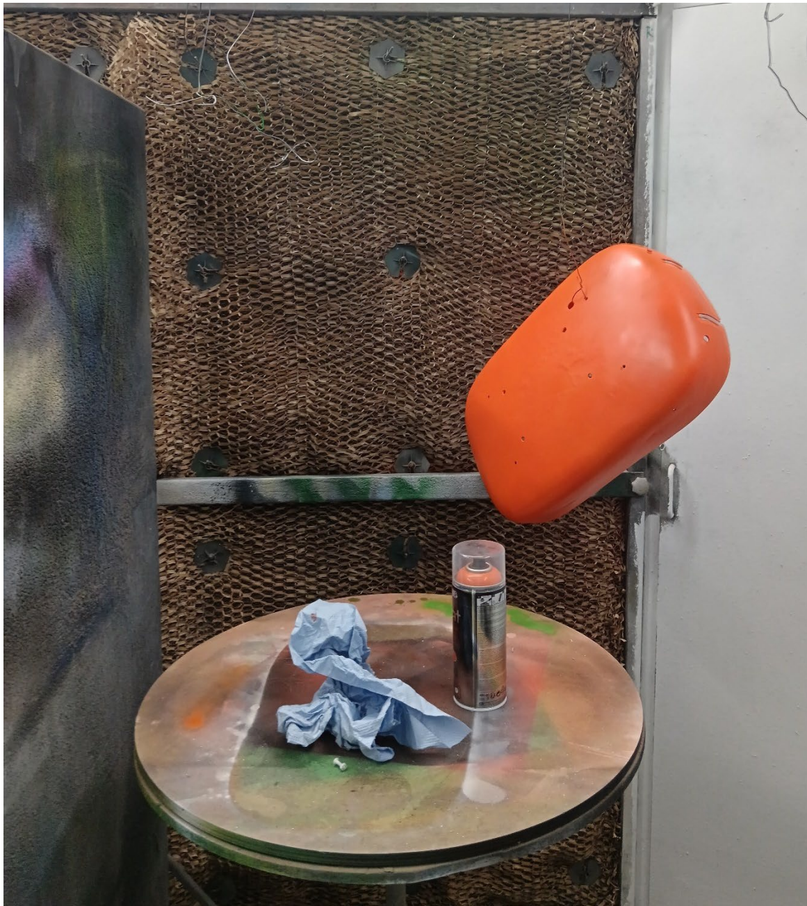
Figure 112: The rear shell was painted with 4 layers of orange spray paint, however it didn't attach well enough to be scratch proof resulting in white marks where the prototype gets scratched.
