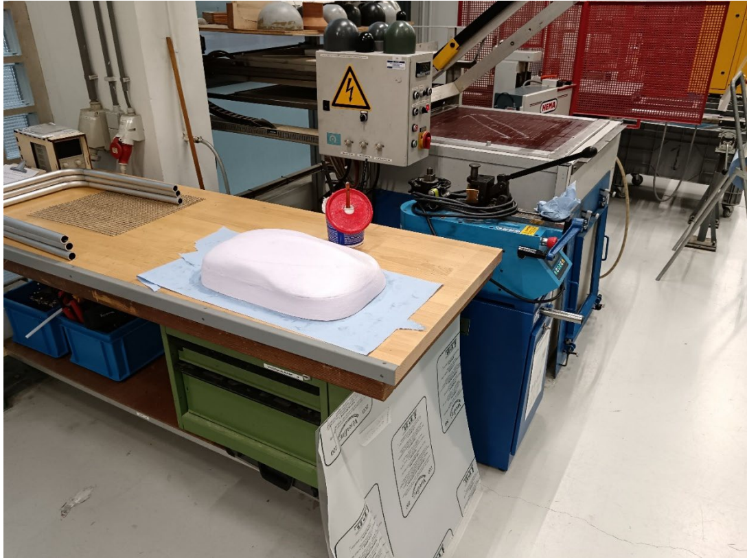
Figure 83: The manufacturing process - Plastered and polished foam model of the frontal lid being covered in Vaseline to be used as a mold for thermoforming.
