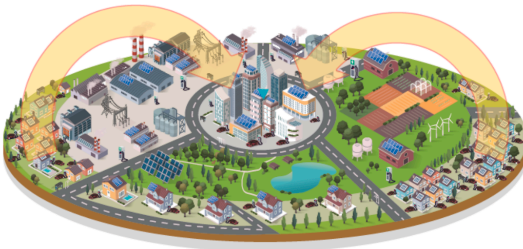
Fig. 1. Conceptual illustration of a SolarEV City. Rooftop PV and EV batteries meet urban electricity demand through coordinated charging, discharging, and local energy exchange. The two arrows represent electricity flows from surrounding suburban areas to urban demand centers through aggregated rooftop PV and EV resources operating as virtual power plants (VPPs).
