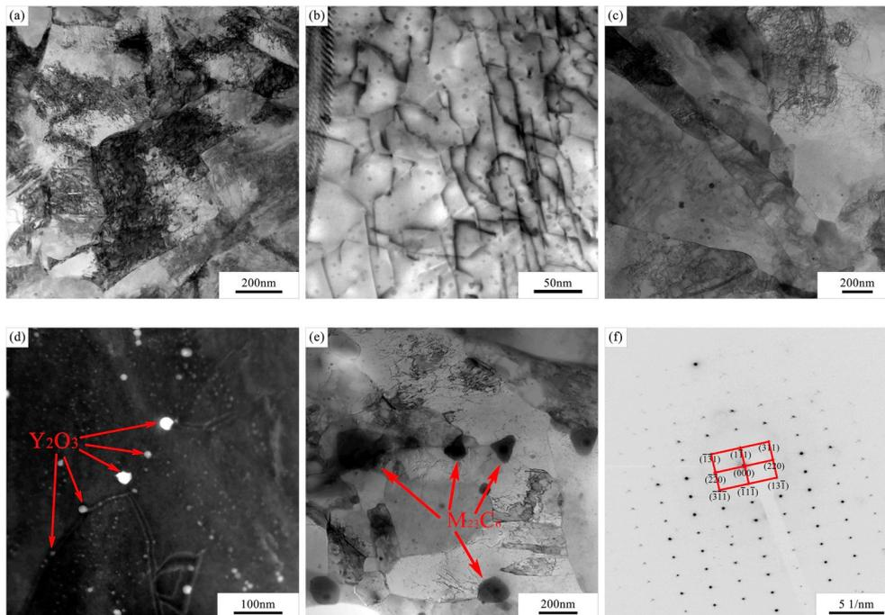
Fig. 9. TEM images of the microstructural features of the (a), (b) as-produced and (c), (d), (e), (f) tempered steel, (a) high density dislocations, (b) homogeneously dispersed  $Y_2O_3$ , (c) tempered martensite lath and clean grains, (d)  $Y_2O_3$  pinning the grain boundaries (e)  $M_{23}C_6$  carbides and (f) diffraction pattern of  $M_{23}C_6$  carbides.
