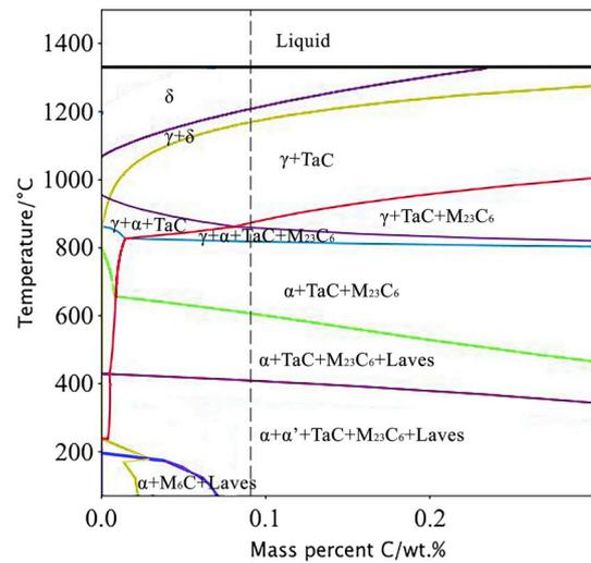
Fig. 8. Computed phase diagram with respect to the carbon content for Fe-9Cr-1.1W-0.4Mn-0.2V-0.12Ta-0.3Y<sub>2</sub>O<sub>3</sub> (wt%).
