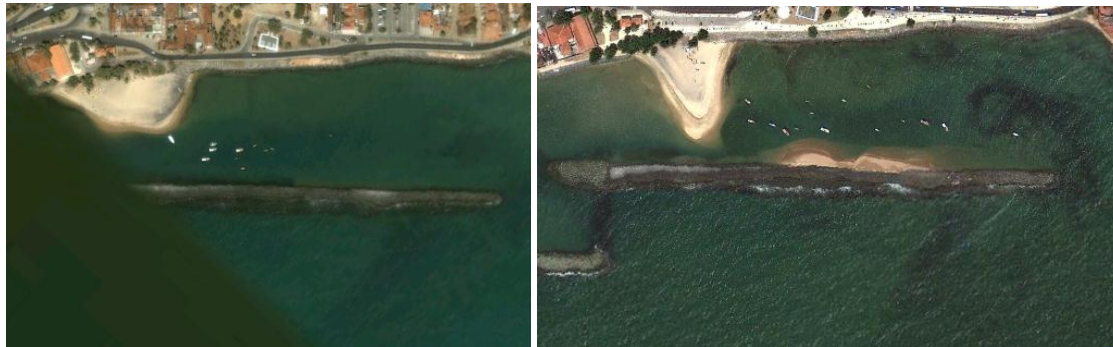
Figure 52: Salient at breakwater A in 2003 (left) and 2010 (right) (Google Earth)
