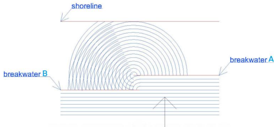
Figure 54: Schematized diffraction pattern between breakwater A and B
