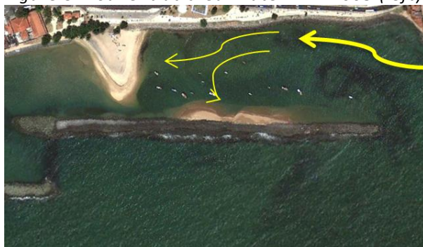
Figure 53: Transport of sediment at breakwater A
