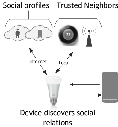
Figure 4.13: Future of DSDN, where trusted devices assist each other. That is, a constrained device delegates authorization to an unconstrained trusted device of the same owner. Thus, the delegation architecture becomes more robust and preserves interaction privacy. Moreover, in general Internet dependency is fully relieved.
