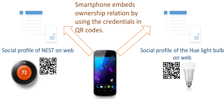
Figure 4.1: The resource owner declares the ownership just by scanning a QR code or RFID/NFC tag that contains the security credentials to update the social profiles of the devices. No other action is required by the resource owner for securing the deployment.
