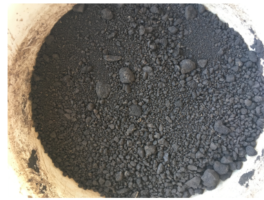
Figure 5.6: Fines remaining after Test 1 and dried in the furnace
