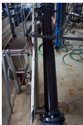
Figure 5.10: Dark water after a few rotations of the batch in the Abrasive Wear Tester
