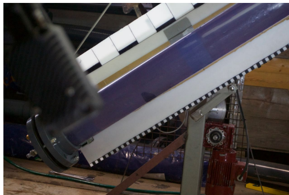
Figure 4.4: The Abrasive Wear Tester with the moving high speed camera, whereas the sliding nodule can be seen, slightly left from the middle of the picture
