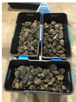
Figure 2.13: Sample of manganese nodules from the CCZ, available for this Master Thesis
