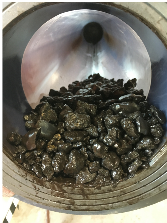
Figure 5.16: The batch of Kinderdijk nodules inside the Abrasive Wear Tester after Test 2
