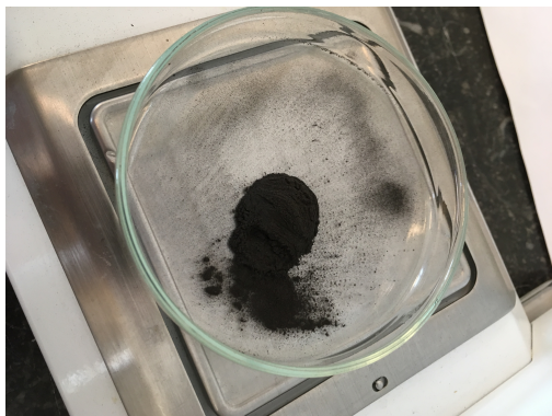
Figure 5.7: Sieved fines on the analytical balance at the MTI laboratory (45 \mu\text{m} )
