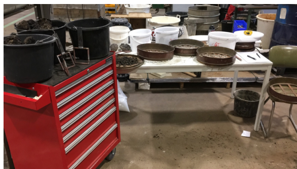
Figure 2.14: Sieving of the manganese nodules at the MTI laboratory in Kinderdijk
