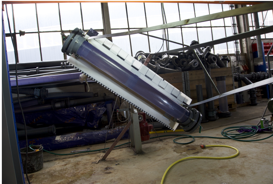
Figure 4.2: Picture of the Abrasive Wear Tester at the MTI laboratory
