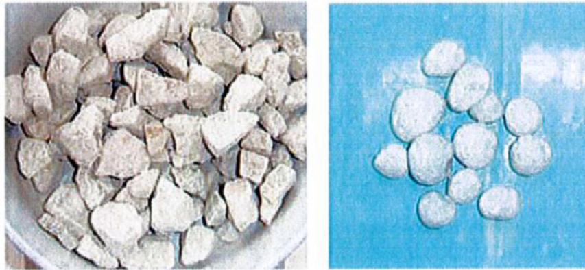
Figure 3.1: Example of particle degradation during slurry transport ( Van den Berg and Alvarez Grima, 2006 )
