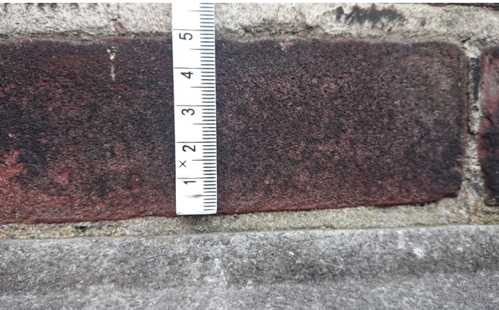
photo 2: height of a stone is aprox. 50mm
