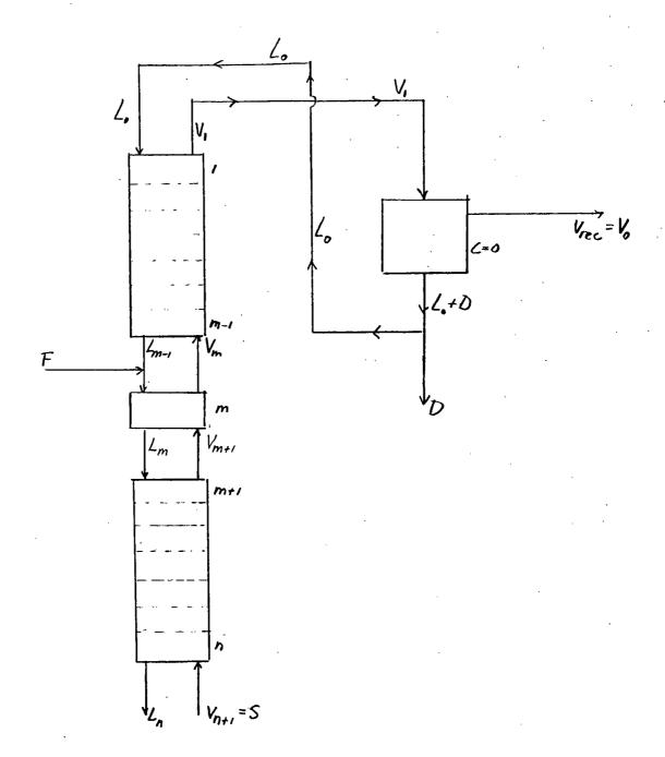
Figure III: Flowsheet for the extraction column with reflux. A scheme for the system built up in four sections. See text for elucidation.
