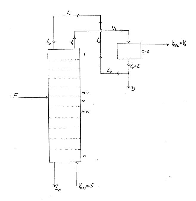
Figure II: Flowsheet for the extraction column with reflux.
