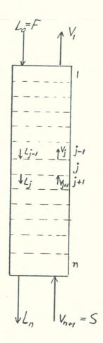
Figure I: Flowsheet for the extraction column without reflux.
