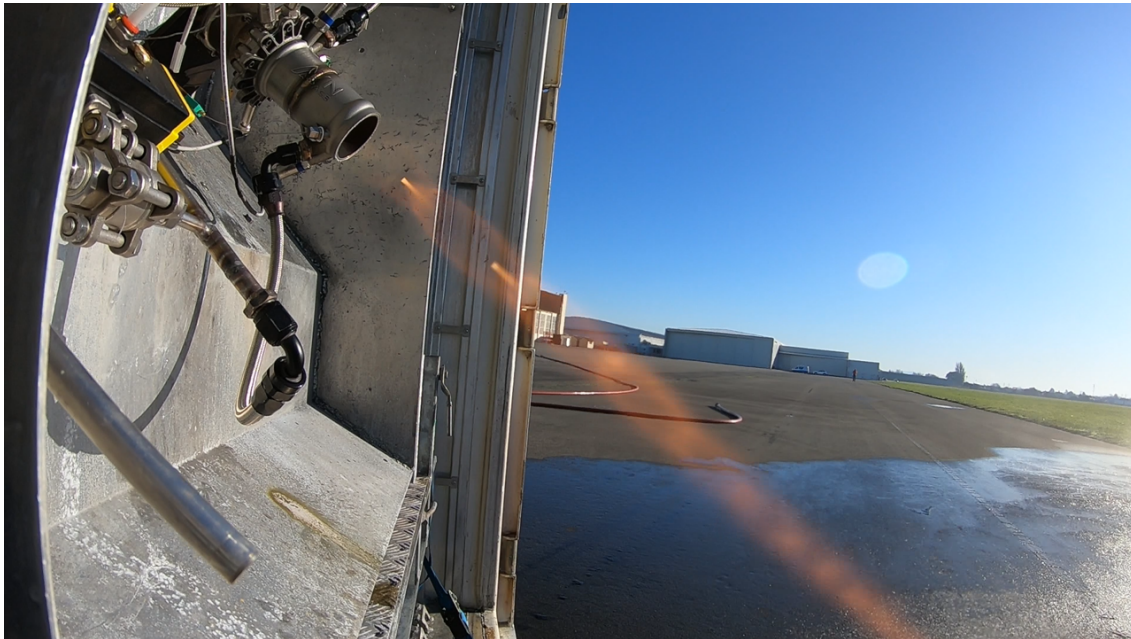
Figure 4.12: Hot-fire test of the Mk-II thruster at the test facility in New Zealand.
