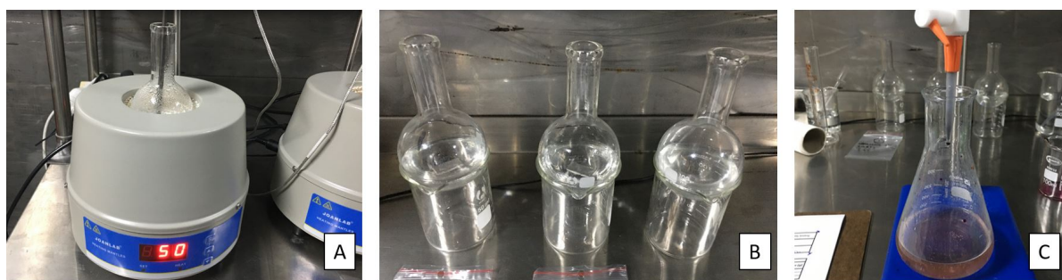
Figure 4.19: Laboratory setup used for immersion screening tests. A) Laboratory heater with boiling flask and thermometer. B) Boiling flasks with passivated and unpassivated test article immersed in hydrogen peroxide, as well as control group. C) Titration of a hydrogen peroxide sample with potassium permanganate.
