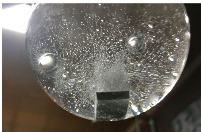
Figure 4.21: Immersion screening test with AM Inconel 718 at 343 K, showing boiling-like phenomena.
