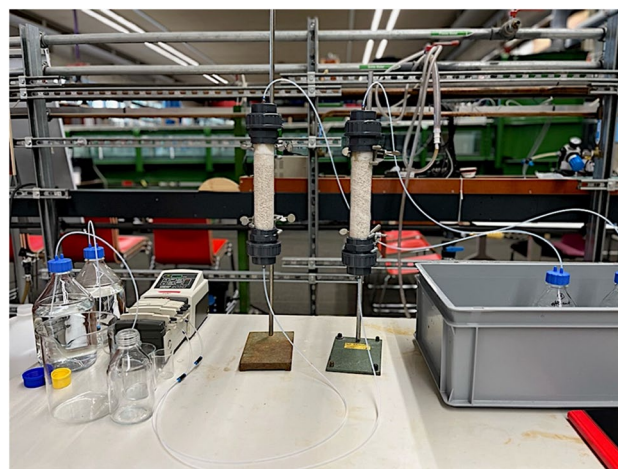
Fig. 2 Experimental setup for leaching tests
