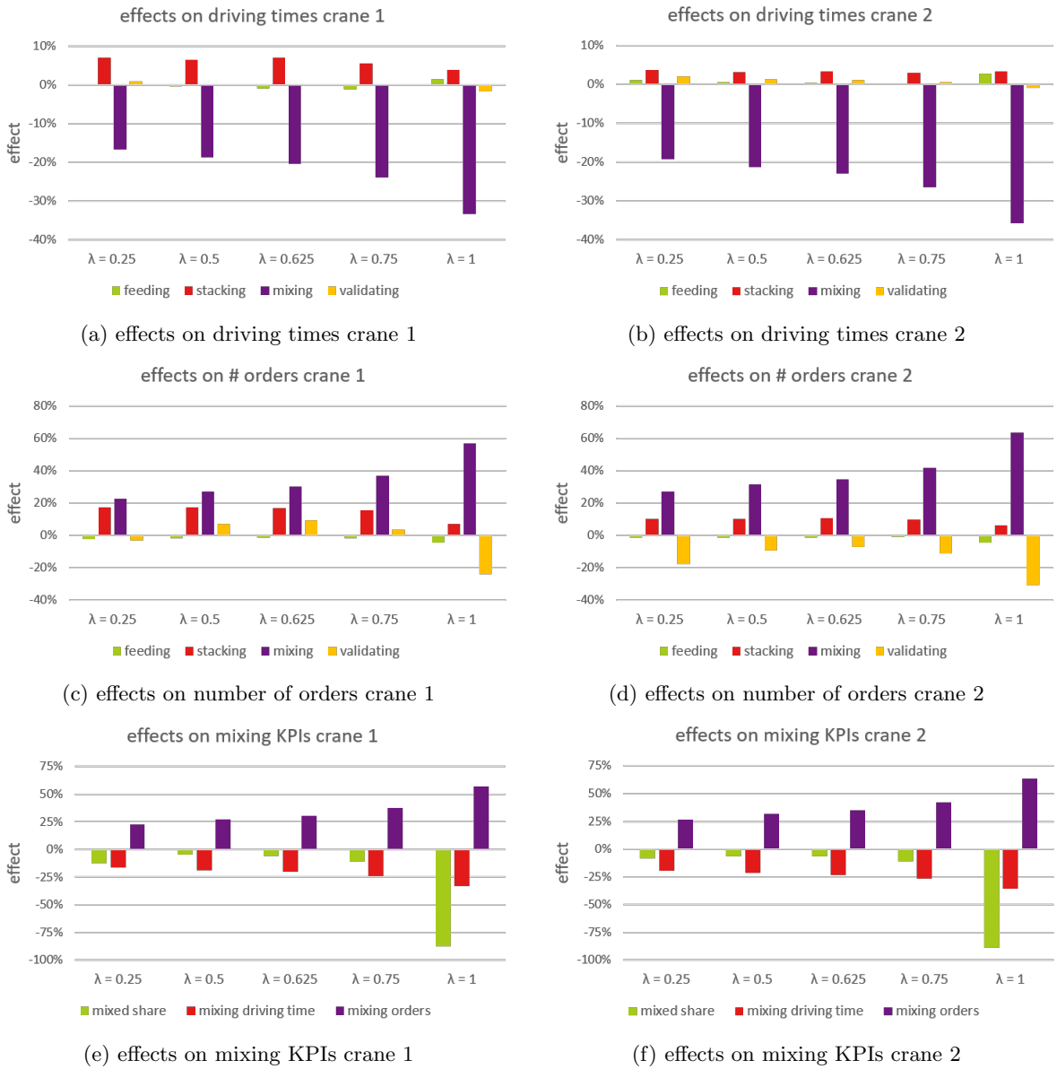
Figure 7.2: Effects of decision rule 3, relative to \lambda = 0 , on driving times, number of orders and mixing KPIs for several values of location scoring weight factor \lambda , based on 20 replications.
