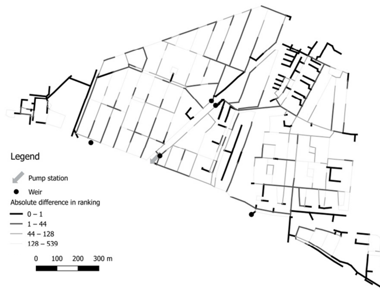
Figure 4.19: Difference in criticality rank between the HMM and the GTM for 'Tuindorp'. The classification of the groups is based on the equal count method.
