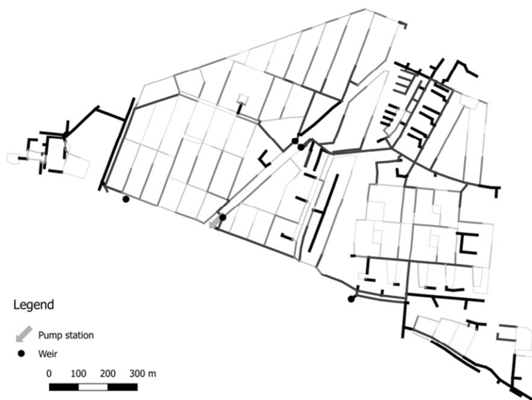
Figure 4.17: Degree of criticality of 'Tuindorp'. The darker the lines the more critical the conduits.
