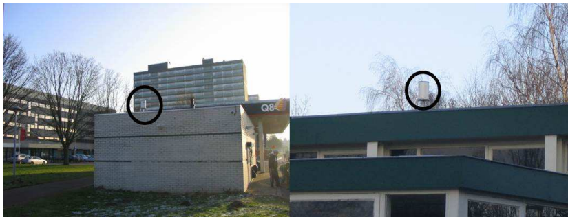
Figure A.2: Locations rain gauges R1 ‘Q8 petrol station’ (left) and R2 ‘Primary school De Regenboog’ (right) in the ‘Tuindorp’ sewer catchment. Installation of the gauges followed the guidelines. There are no obstructions affecting the measurements.
