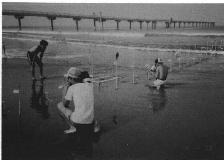
Photo 2 Measurement for the bottom surface level using video movie cameras.
