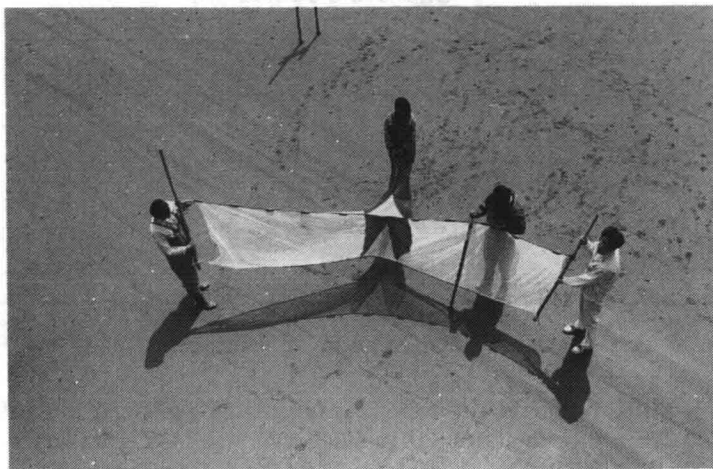
Figure 3 Photograph of net sampler
