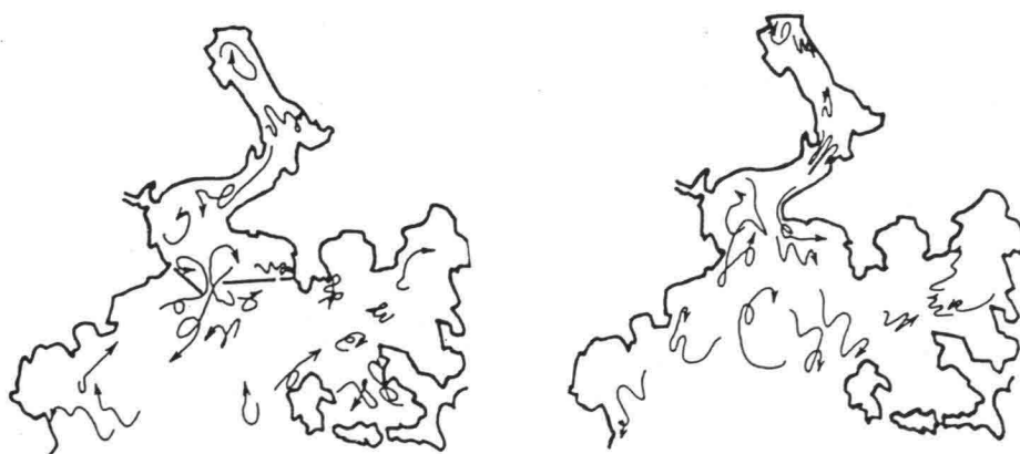
Fig.6(a) Float trajectories for 2 tidal cycles. (with breakwater without density current) Fig.6(b) Float trajectories for 2 tidal cycles. (without breakwater without density current)
