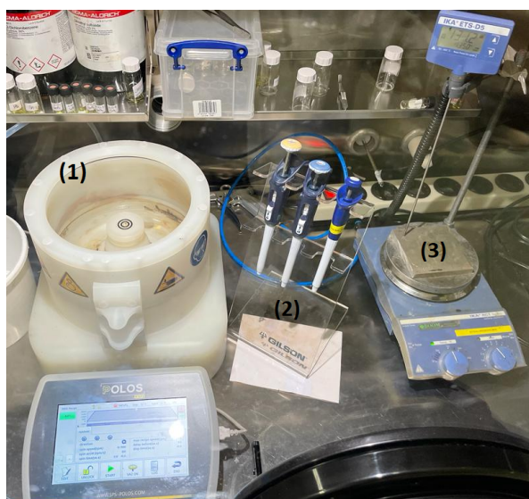
Figure 3.9: Spin-coating setup with (1) Polos spin-coater, (2) pipettes and (3) hot plate.
