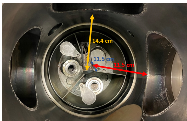
Figure 4.2: Top view of the evaporation chamber with distances between the sensor and sensor walls indicated after optimisation. The yellow arrow represents the distance between the sensor and the middle of the back wall, the red arrow represents the distance between the right side of the sensor and the right chamber wall and the blue arrow represents the height of the top left corner of the sensor to the metal shield separating the source areas.
