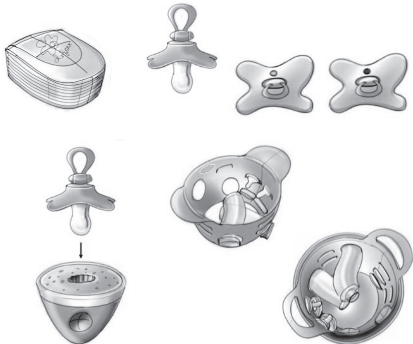
Some of the developed concepts for hygiene at home and on the road: a steriliser and a cleanliness indicator on a pacifier.
