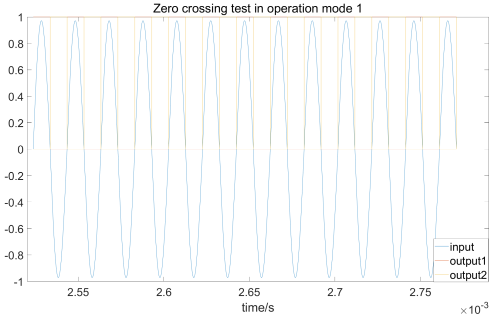
Figure 3.5: Input and output of zero crossing in operation mode 1
