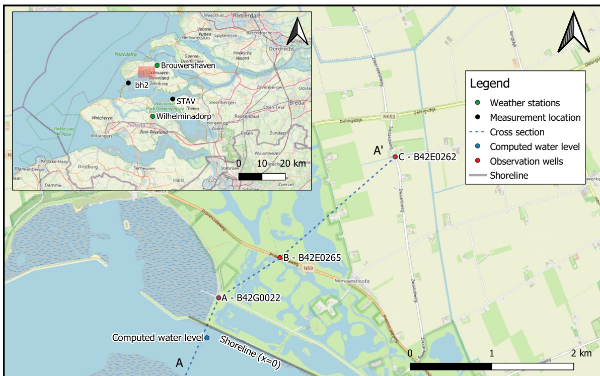
Figure 2.1: Map of the study area (marked transparent red in the small overview map), with the measuring points of the astronomical tide (black dot), weather stations, with location from cross Section of Figure 2.2 & 7.1
