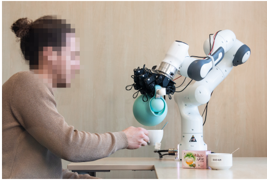
Fig. 1. Example of an embodied human-robot interaction: Here a robotic arm collaboratively making tea with the person. Such a task involves both cognitive interaction and force exchange on the physical level.
