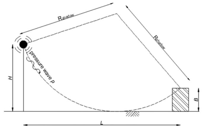
Fig. 5. Graphical representation of the shadow zone resulting from the curvature of the sound waves.
