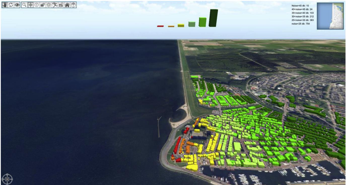
Fig. 13. Wind turbine noise propagation in Test Case 1.
