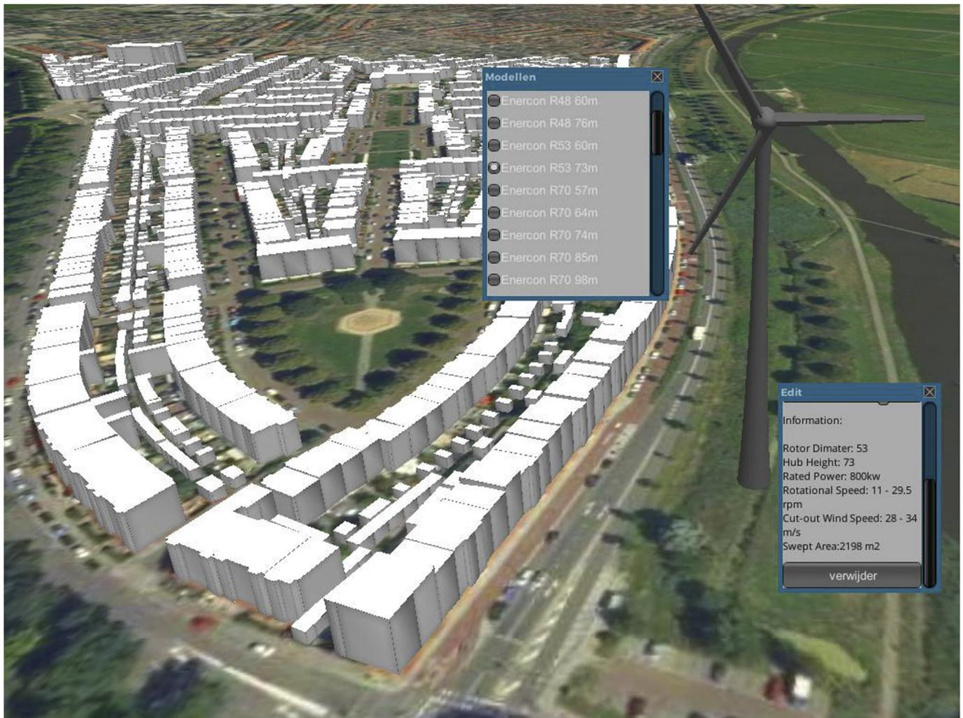
**Fig. 7.** Wind turbine scenario design in Falcon. Users can select different wind turbine types and bring them into the scene as game objects. By placing a wind turbine in the scene, its geometric and technical characteristics are retrieved from the database and are presented.
