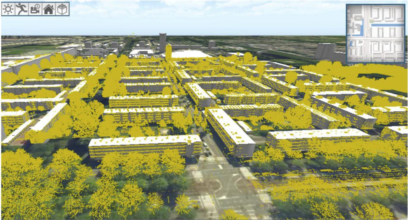
**Fig. 6.** AHN2 LIDAR point cloud overlaid on 3D models in Falcon. Different 3D and 2D geospatial data of the whole Netherlands are served to Falcon via web services.
