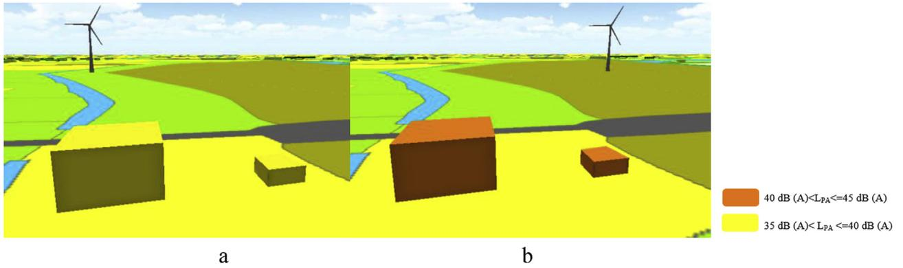
**Fig. 8.** Placement of the wind turbine on different land-use types leads to different noise being received on the same buildings: a) grass field and b) arable land. All other parameters (e.g. wind turbine-building distance) remain the same.
