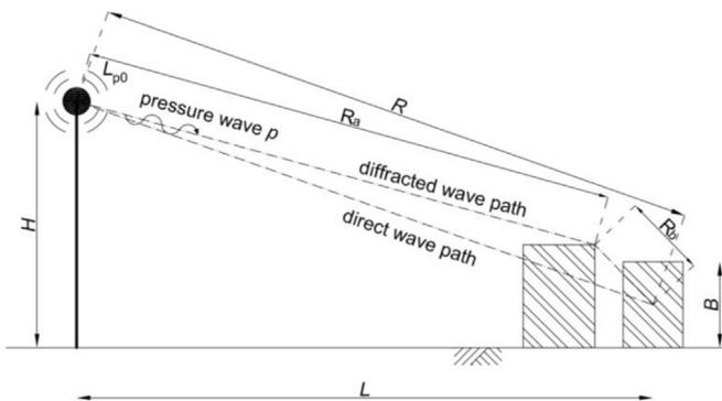
Fig. 4. Graphical representation of the direct and diffracted wave.
