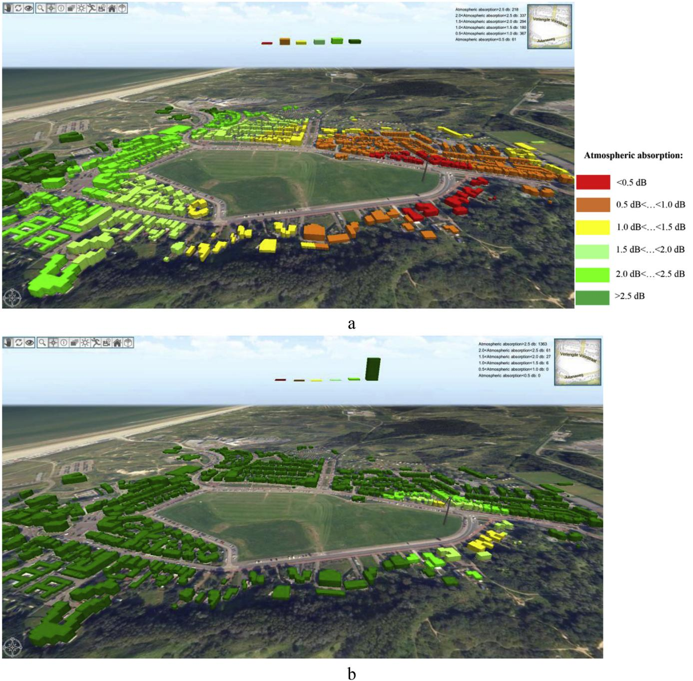
Fig. 10. Implementation of atmospheric absorption sub-module for a) current humidity situation estimated by hourly humidity data (80.6%) and b) adjusted humidity (20%).
