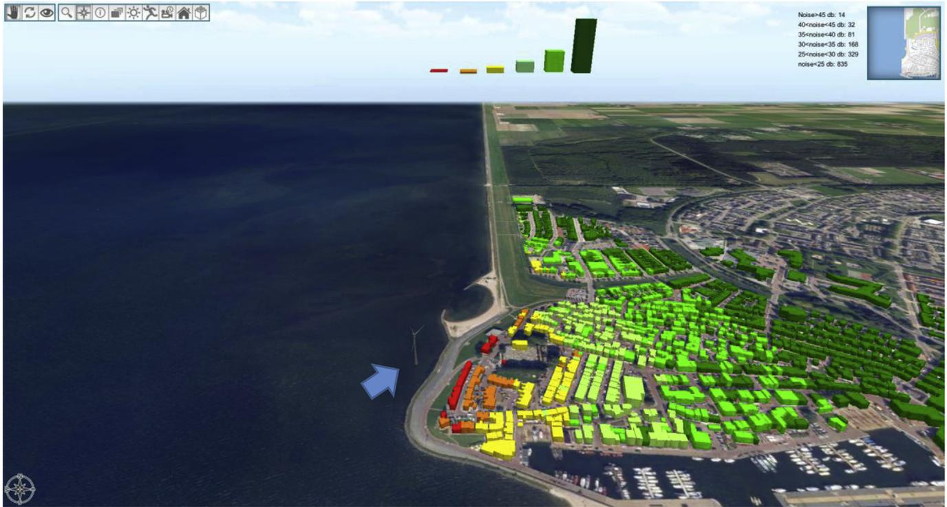
Fig. 14. Wind turbine noise propagation in Test Case 2.
