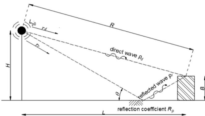
Fig. 2. Graphical representation of the direct and reflected wave.
