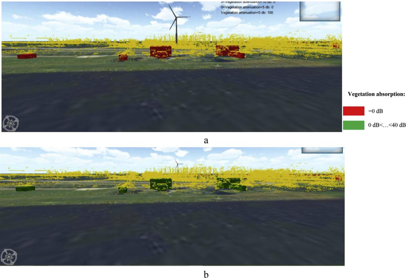
**Fig. 9.** Sound attenuation due to vegetation (sound frequency is set to 1000 HZ) depicted in two scenarios. By placing the wind turbine further from the target buildings from scenario a to b the number of buildings affected by line-of-sight obstruction by the forest increases.
