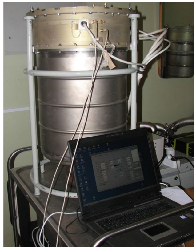
Fig. 3. One of the RadioAstron's on-board H-maser units undergoing laboratory tests, Moscow, Astro Space Center of P.N. Lebedev Physical Institute, July 2008.
