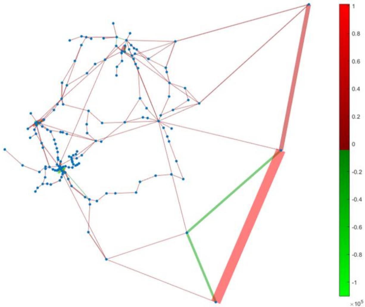
Figure 6.16: Visualization of differences in passenger flow intensities on PT links between initial state and final state for Randstad PT network
