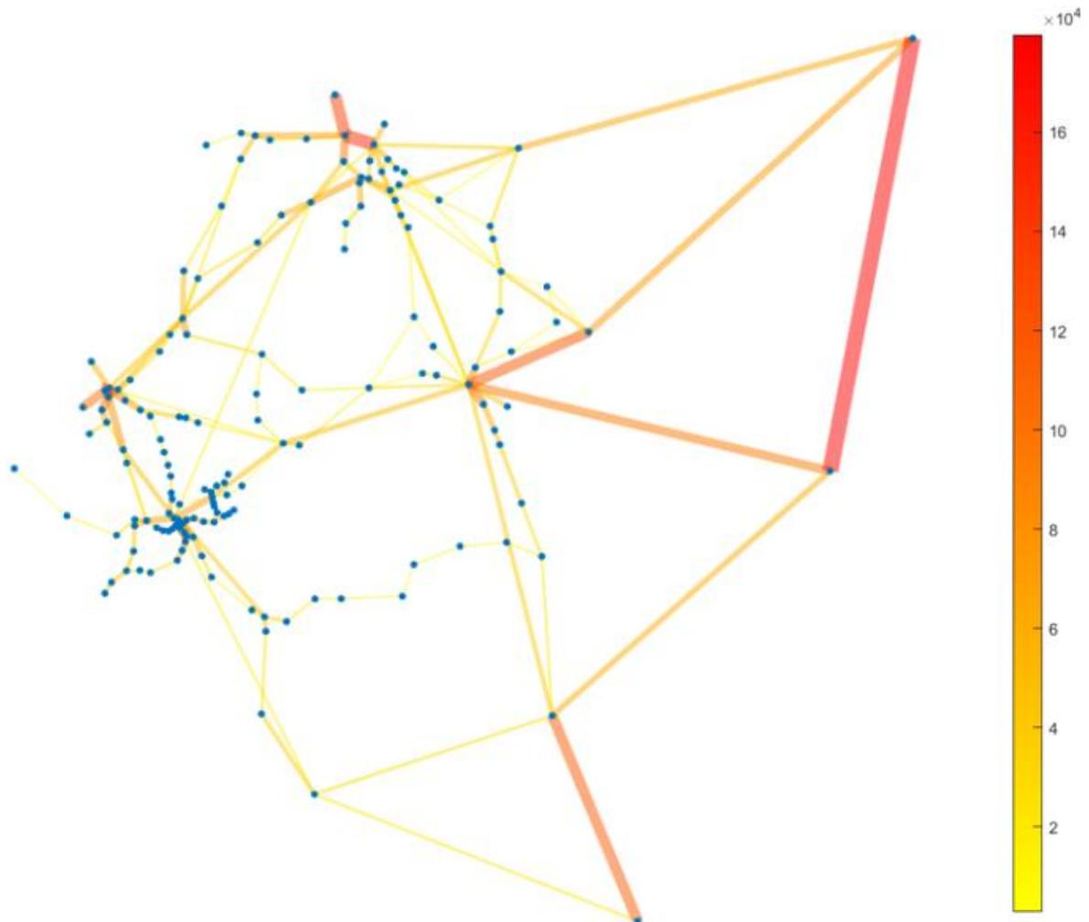
Figure 6.7: Visualization of passenger flow intensities on PT links in initial state for Randstad PT network
