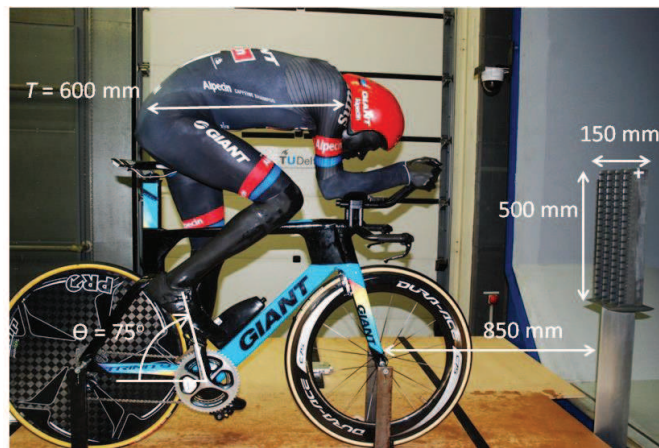
Fig. 2 Wind tunnel model and PIV seeding system.
