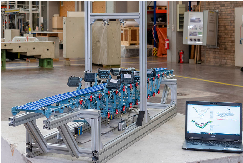
Figure 4.1: Small scale model of a cable-stayed truss bridge, constructed in 2024 by BAM and TNO [51].
