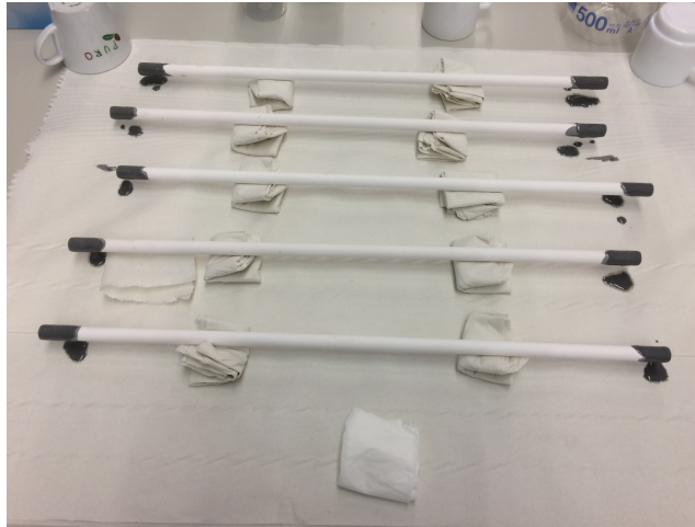
Figure 4.1: Application of Epoxy glue on the edges of the tubular membranes
