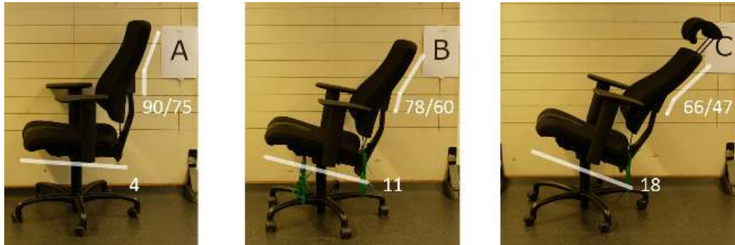
Figure 3 Three different sitting positions (A, B, C) for the seat and back rest
