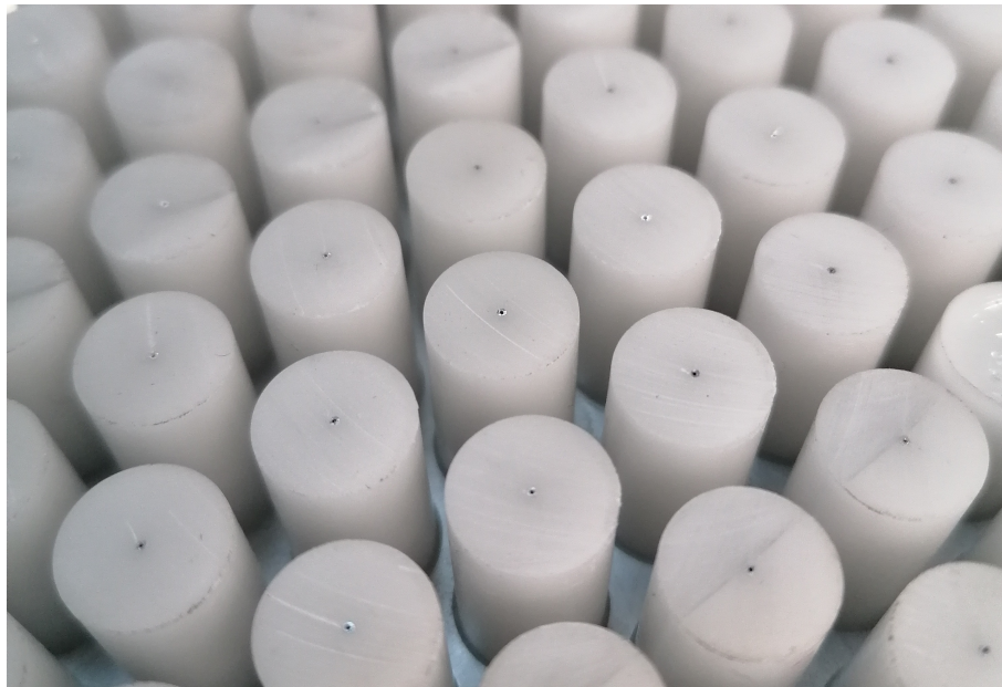
(b) Scratches are still visible in the surface of the pins, however, these will be removed after sanding. Some needles are partly closed due to a burr that is created during the machining operation. This burr is also removed during the sanding process.
