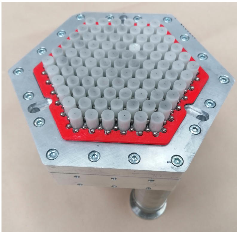
(b) The plenum chamber is sealed by the plenum lid using socket head cap screws ( 18 \times M5 \times 25 ). The outer ring of balls is kept in place using a 3D ball constrainer.
