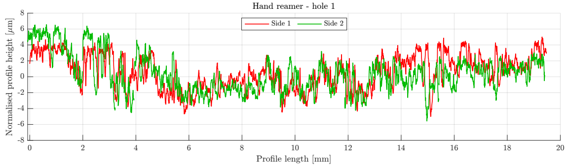
(b) Surface profile for hand reamed surface (close-up).
