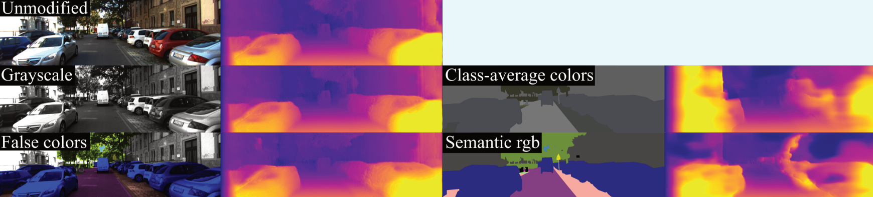
Figure 8. Removing color information or even replacing it by false colors does not significantly affect the depth estimate. Removing the texture, however, leads to significantly worse results.
