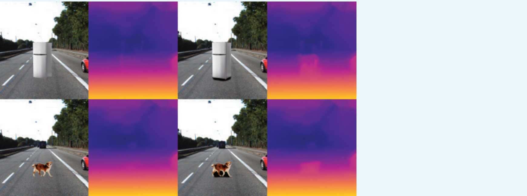
Figure 10. Objects that do not appear in the training set can be detected, but only when a dark shadow is present along their bottom edge.
