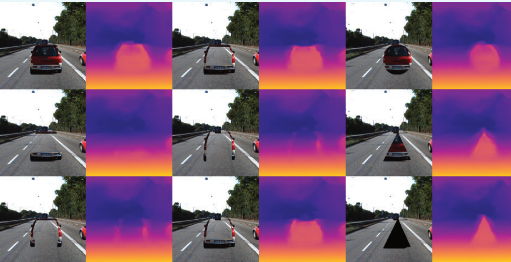
Figure 9. Not all parts of the object are required for detection; Monodepth can still recognize cars when their outline is present. Obstacles do not need a recognizable shape nor texture to be detected.
