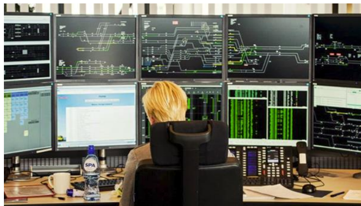
Figure 6: Workstation of a train traffic controller in the Netherlands.
