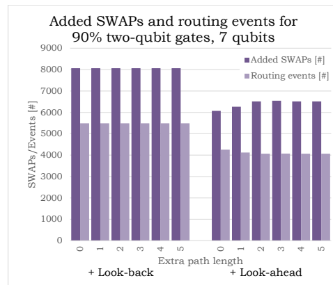
Figure B.16: Number of routing events and added SWAPs for different extra path lengths to allow detours. The random benchmark contains 90% two-qubit gates for 7 qubits.
