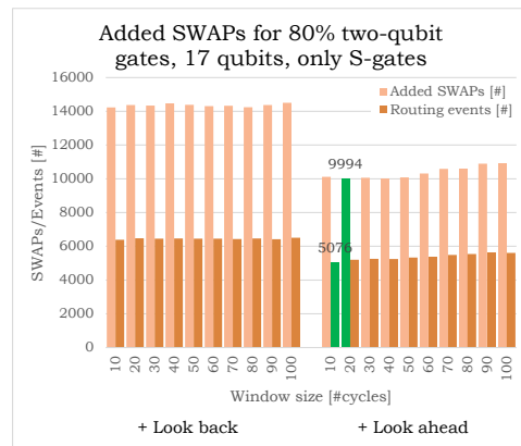
Figure C.20: Number of routing events and added SWAPs. The random benchmark contains 20% S-gates and 80% two-qubit gates for 17 qubits.
