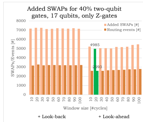
Figure C.8: Number of routing events and added SWAPs. The random benchmark contains 60% Z-gates and 40% two-qubit gates for 17 qubits.
