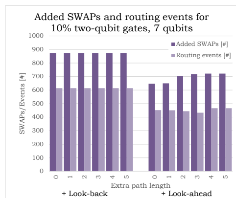
Figure B.2: Number of routing events and added SWAPs for different extra path lengths to allow detours. The random benchmark contains 10% two-qubit gates for 7 qubits.
