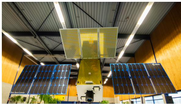
Figure 2.10: The M-Argo CubeSat in its deployed configuration [19].
