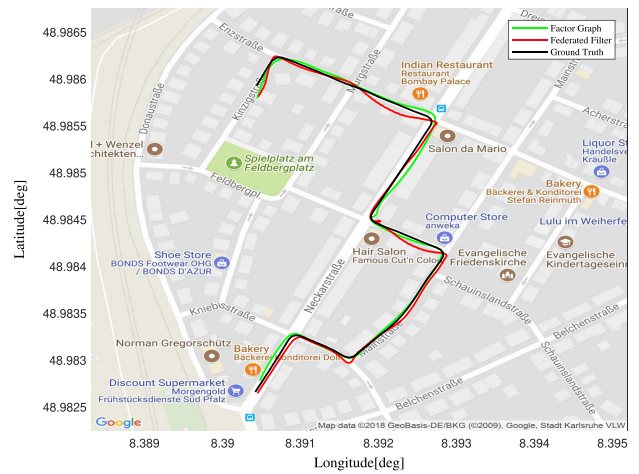
FIGURE 7. Trajectories for the ground truth, factor graph method, and Federated Filter on KITTI dataset.
