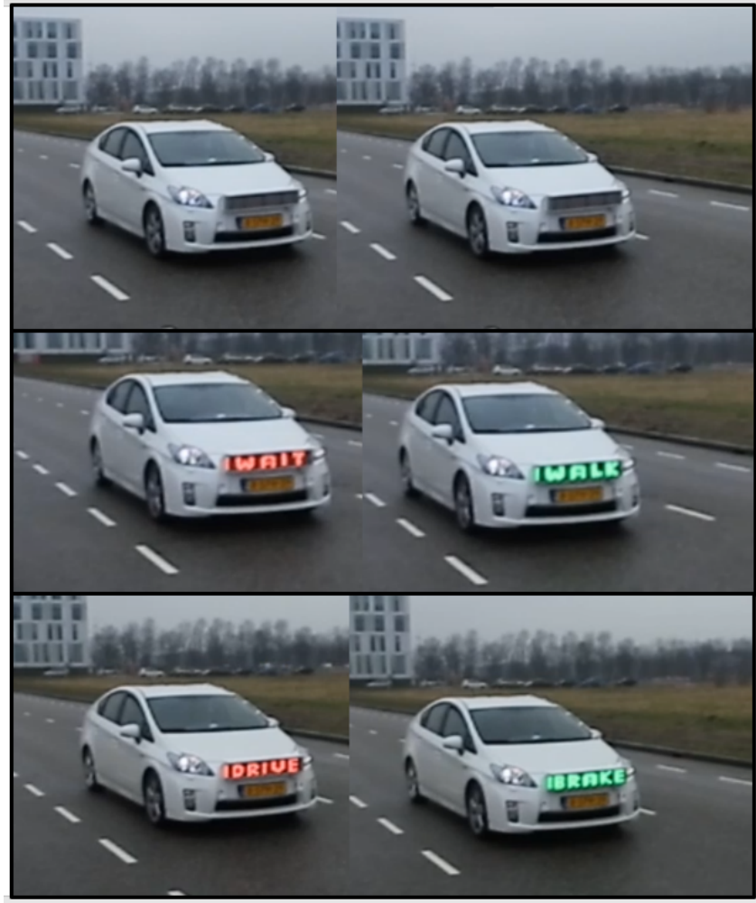
Figure 2.5: Information type \eta as shown on the eHMI in the real environment, with non-yielding state ( left ) and yielding state ( right ). From top to bottom: (1) None: Baseline condition, no information displayed, (2) WAIT/WALK: Egocentric, advisory information, (3) DRIVE/BRAKE: Allocentric, vehicle-based information.
