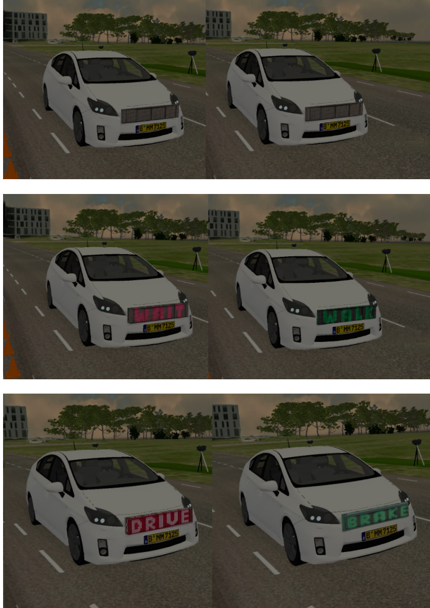
Figure A.2: Information type \eta as shown on the eHMI in the virtual reality environment, with non-yielding state ( left ) and yielding state ( right ). From top to bottom: (1) None: Baseline condition, no information displayed, (2) WAIT/WALK: Egocentric, advisory information, (3) DRIVE/BRAKE: Allocentric, vehicle-based information.
