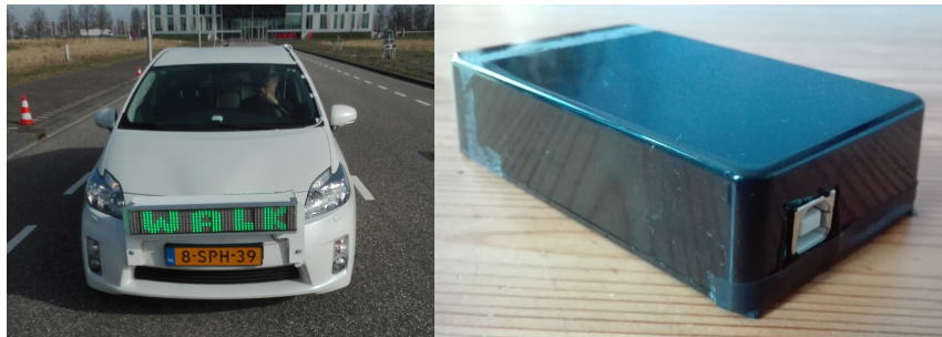
Figure A.1: Left : Example of the eHMI showing a WALK message. Right : The GPS module as packed in a small black box with the USB-B connector visible.
