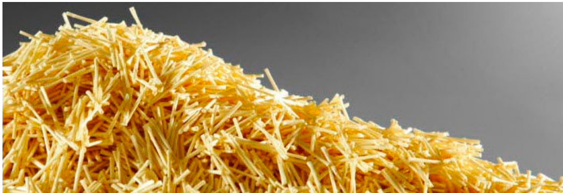
Fig. 2.5 - Close-up of chopped aramid fibres [Source: http://www.directindustry.com/pt/prod/teijin-aramid/roduct-18087-1097033html ]
