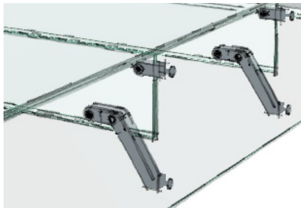
Fig. 4.27 - Connecting brackets between the main beam and the cross beams. The amount of steel was minimized due to FEM analysis. [Krynski et al., 2012]
