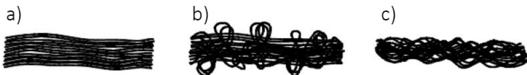
Fig. 2.7 - Different types of rovings: a) smooth roving b) interlaced roving c) tangled roving [Potyrala, 2011]
