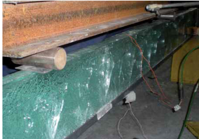
Fig. 5.4 - Bending test with structural glass beam. [Speranzini et al., 2011]
