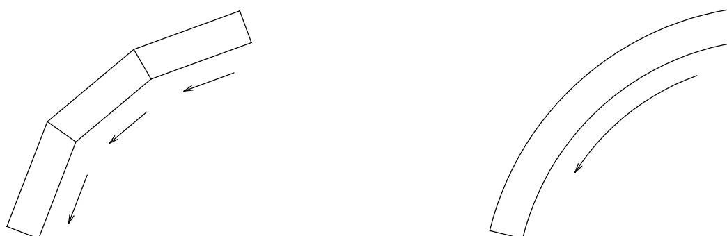
Fig. 7.11 - The gridshell has continuous curvature while the lattice structure and the plate shell are discrete leading to bending moments between the facets.
