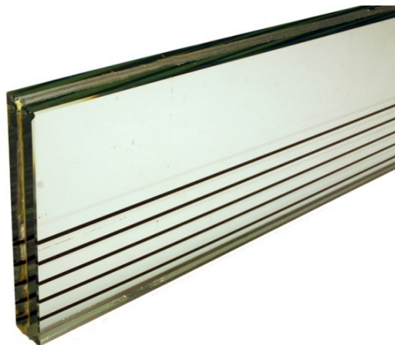
Fig. 5.1 - Test specimen of the structural glass beam with rounded glass fibre rods embedded in the glass sheets [Louter, 2010]
