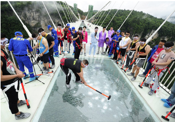
Fig. 4.17 - Destruction of the laminated glass panels with sledgehammers to demonstrate the safety of the bridge [Source: https://www.thestar.com/news/world/2016/08/03/china-opens-terrifying-tianmen-mountain-glass-walkway.html ]
