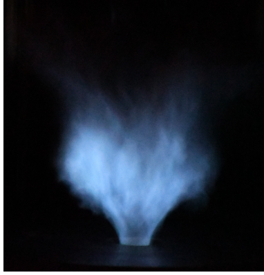
Figure 6.1: DSLR picture of ref. flame (P:8 kW, H 2 : 25%, AAI:10%)
