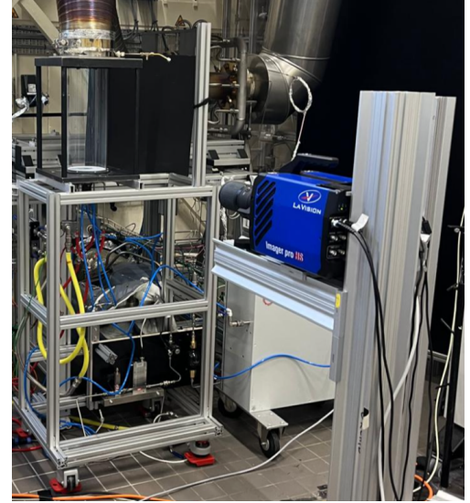
Figure 5.12: LaVision imager HS Pro pointed at setup
