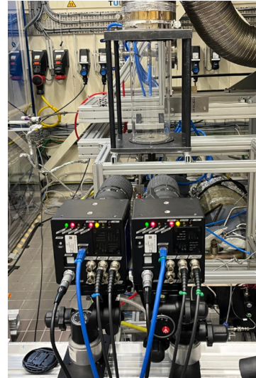
Figure 5.14: Side-by-side Photron fastcams capturing the set-up
