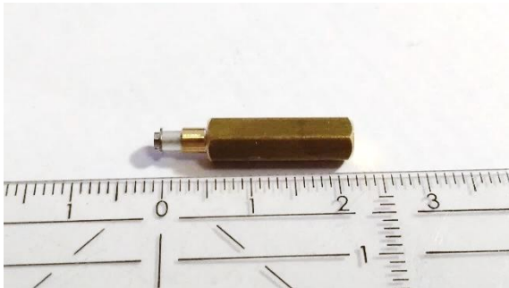
Figure 35: Compression tool with the opaque white PUR(r) spring inserted on the left
