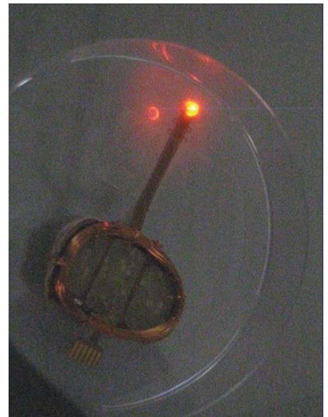
Figure 7: Wireless PDT device for brain implants.
