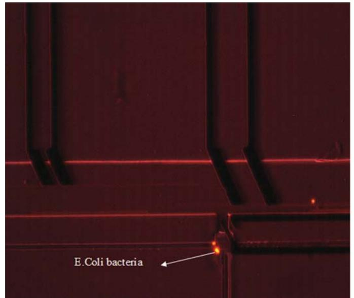
Figure 8 (left) Optical waveguide for detecting E-coli (right) microchannels for isolating e-coli for further analysis
