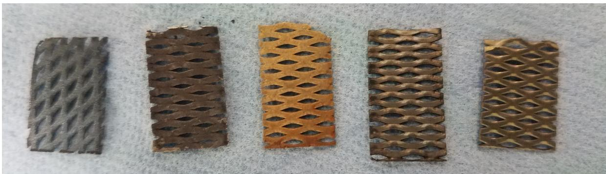
Figure G.5. Electrode fragments for XPS analysis. From left to right: Permascand, RNi, NiFe-LDH, NiFe and Nickel mesh.
