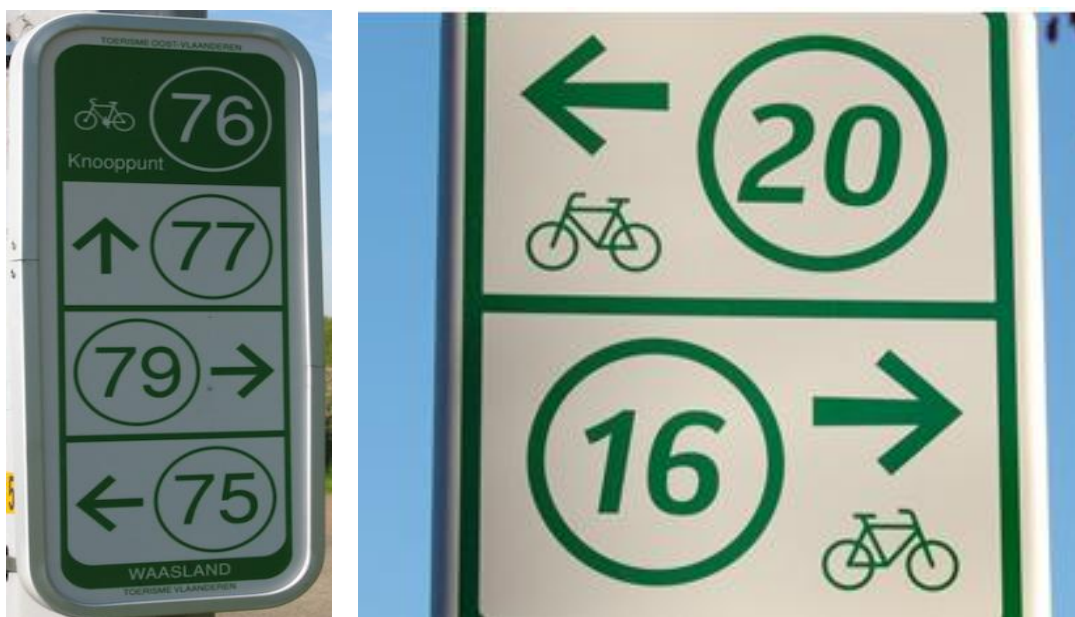
Figure 3.2: Signage of Junction Network System
