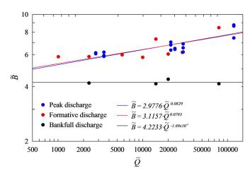
Figure 12 Dimensionless width versus dimensionless discharge. Black dots and black trend line: width versus geometrical bankfull discharge. Red dots and red trend line: width versus constant formative discharge. Blue dots and blue trend line: equilibrium width versus peak discharge (variable discharge cases)
