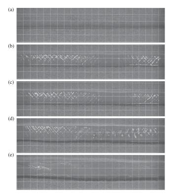
Figure 5 Channel width evolution with sediment S4 (D<sub>50</sub> =  $1.0 \times 10^{-3}$  m) and discharge hydrograph H3 at: (a) T = 0 min (B = 0.093 m), (b) T = 15 min (B = 0.105 m), (c) T = 30 min (B = 0.107 m), (d) T = 60 min (B = 0.137 m), and (e) T = 150 min (B = 0.153 m). The flow conditions are listed in Table 3 and the hydrographs are shown in Figure 4
