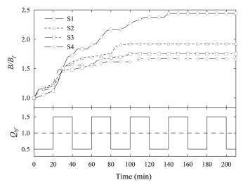
Figure 8 Dimensionless channel-width evolution as a function of time resulting from hydrograph H2 (top) and discharge variation (below) as a function of bankfull discharge
