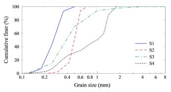
Figure 2 Grain size distributions of the sand samples used in the experiments
