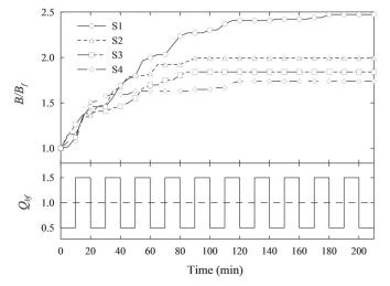
Dimensionless channel-width evolution as a function of time resulting from hydrograph H1 (top) and discharge variation (below) as a function of bankfull discharge
