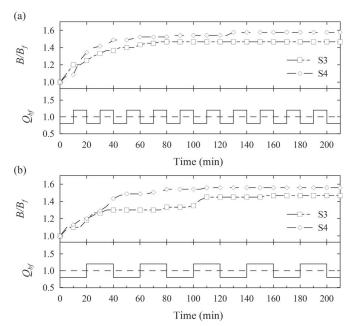
Figure 10 Dimensionless channel-width evolution as a function of time for the sediment samples S3 and S4 with the hydrographs: (a) H4 and (b) H5
