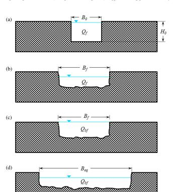
Figure 3 Experimental procedure subdivided in stages (a) 1, (b) 2, (c) 3 and (d) 4  $\,$
