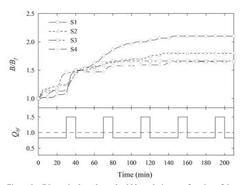
Dimensionless channel-width evolution as a function of time resulting from hydrograph H3 (top) and discharge variation (below) as a function of bankfull discharge
