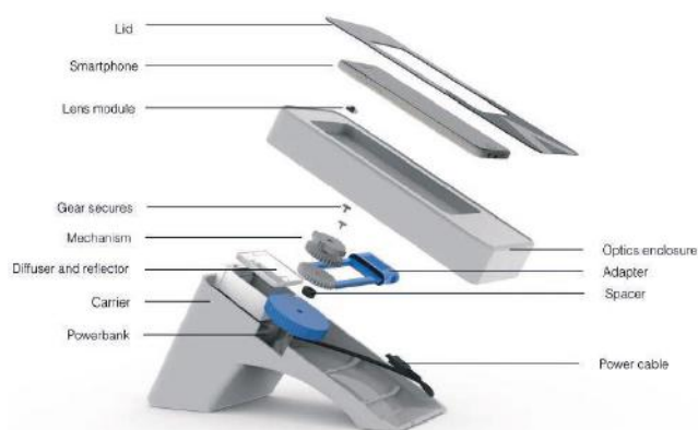
FIGURE 2.1 Exploded view of all elements of the Excelscope 1.0
