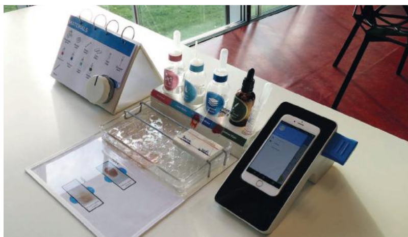
FIGURE 2.3 A prototype of a designed toolkit that supports the healthworker in the staining procedure.
