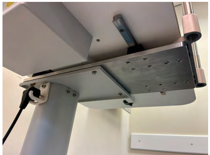
Figure 102, connection piece between stand and the frame
