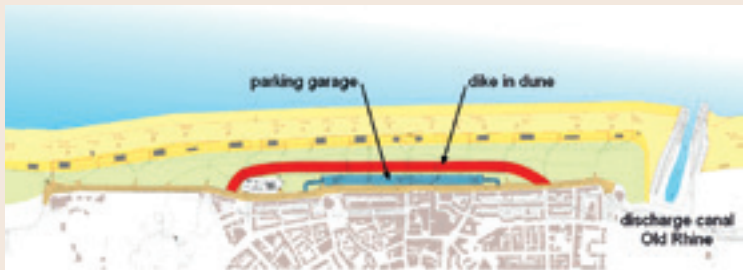
Figure 2 (mid below). Katwijk: overview of the area with location of the dike-in-dune and parking garage. (Kustwerk Katwijk, 2012).
