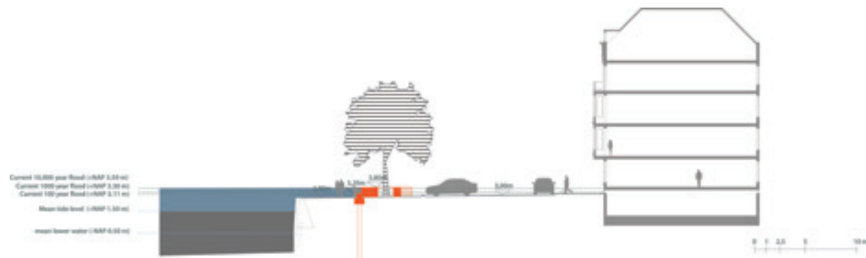
Figure 3. Cross section of Noordereiland: op- tion flood protection by large bench and boulevard (image courtesy Peter van Veelen).
