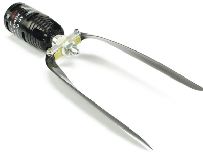
Figure 13.4: Folding Propeller Example
