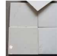
Reclaimed wall tiles
