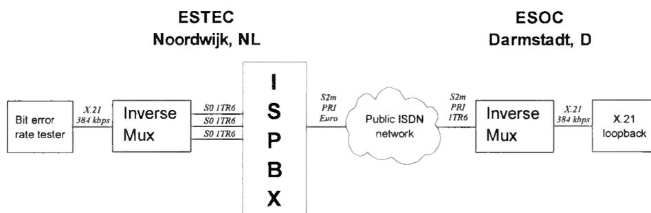
**Figure 3.1** *Test configuration*
