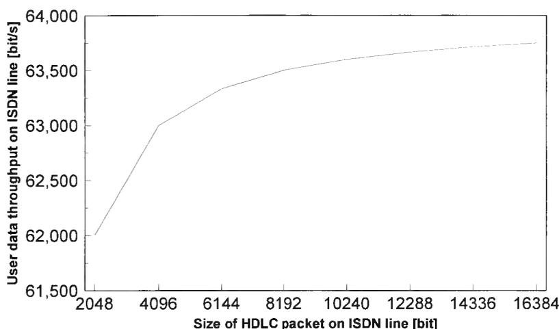
**Figure 6.6** *PC-to-PC file transfer throughput on an ISDN line with HDLC framing.*
