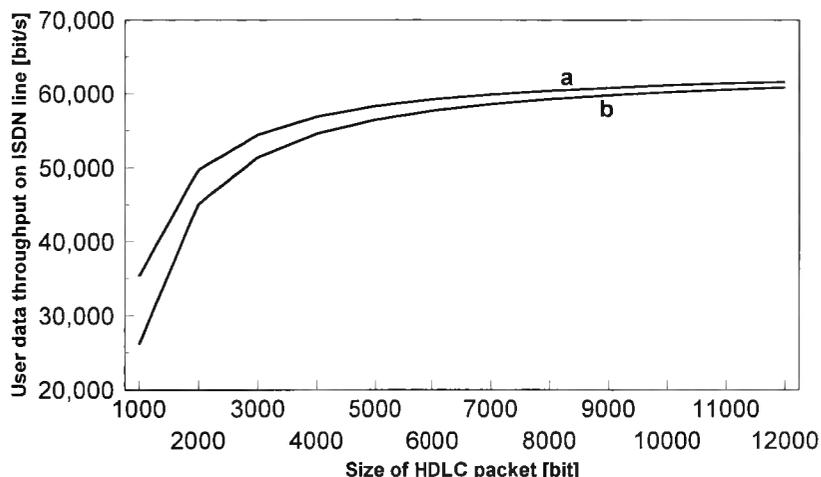
**Figure 6.2** Net user data throughput on a 64 kbit/s ISDN link using Ethernet bridging and routing and TCP/IP protocols as a function of the size of the HDLC packet. (a) routing; (b) bridging.
