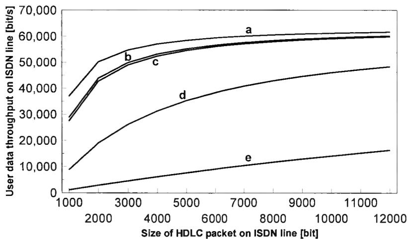
**Figure 6.5** Net user data throughput on a 64 kbit/s ISDN link using Ethernet routing and IPX/SPX protocols as a function of the size of the HDLC packet. (a) burst mode, 1 ACK per 10 SPX packets, no delay; (b) burst mode, 1 ACK per 100 frames, 0.26s delay; (c) stop-and-wait mode, 1 ACK per SPX packet, no delay; (d) burst mode, 1 ACK per 10 SPX packets, 0.26s transmission delay; (e) stop-and-wait mode, 1 ACK per SPX packet, 0.26s transmission delay.
