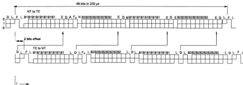
**Figure 2.7** Structure of S/T basic-access frame.
