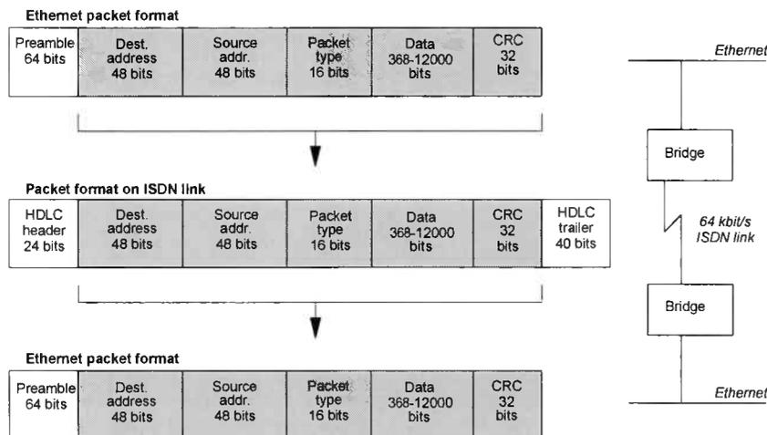
**Figure 6.1** Bridging of Ethernet frames through an ISDN circuit.
