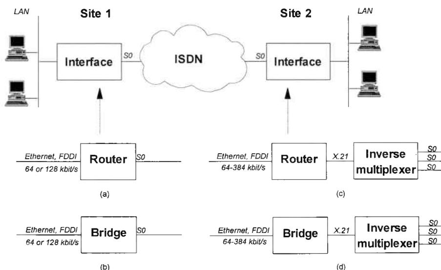
**Figure 5.1** Different options for LAN-LAN links over the ISDN. (a) An ISDN router, (b) ISDN bridge, (c) non-ISDN router, (d) non-ISDN bridge.
