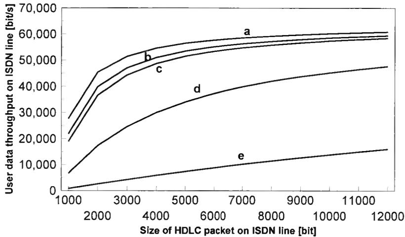
**Figure 6.4** Net user data throughput on a 64 kbit/s ISDN link using Ethernet bridging and IPX/SPX protocols as a function of the size of the HDLC packet. (a) burst mode, 1 ACK per 10 SPX packets, no delay; (b) burst mode, 1 ACK per 100 frames, 0.26s delay; (c) stop-and-wait mode, 1 ACK per SPX packet, no delay; (d) burst mode, 1 ACK per 10 SPX packets, 0.26s transmission delay; (e) stop-and-wait mode, 1 ACK per SPX packet, 0.26s transmission delay.
