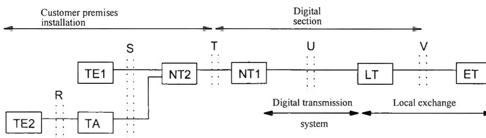
**Figure 2.2** Subscriber-access network reference configuration.
