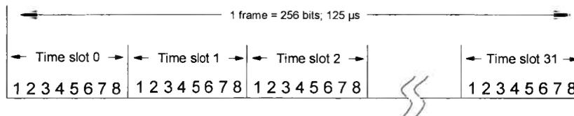
**Figure 2.9** *Structure of S/T 2048 kbit/s primary-access frame*
