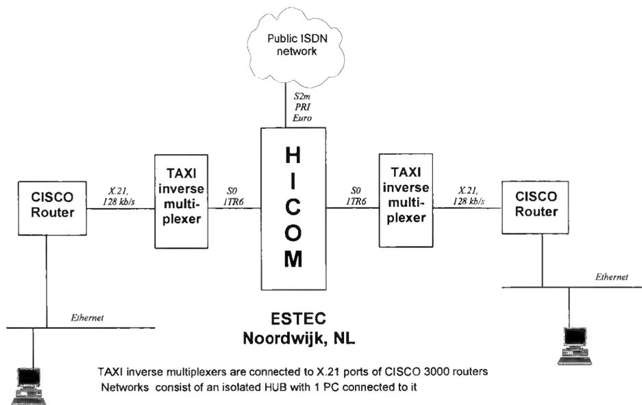
Figure 5.4 128 kbit/s LAN-to-LAN link.
