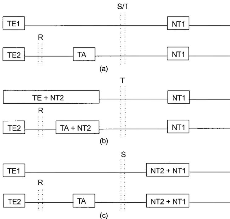
**Figure 2.3** *Point-to-point subscriber-access network reference configurations*
