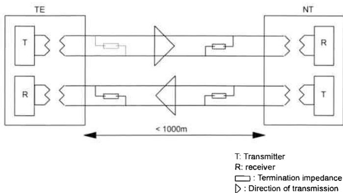
Figure 2.5 Point-to-point wiring configuration
