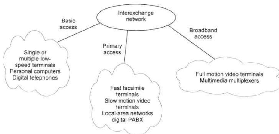
**Figure 2.4** *Basic access, primary access and broadband access*
