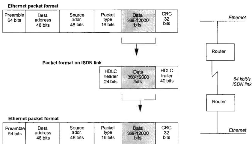
**Figure 6.3** Routing of Ethernet frames through an ISDN line.
