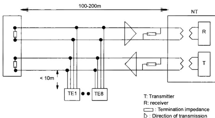
Figure 2.6 Short passive bus wiring configuration
