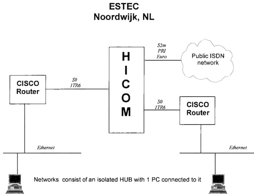
Figure 5.3 64 kbit/s LAN-to-LAN link
