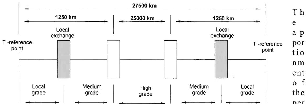
**Figure 3.2** Circuit quality demarcation of longest hypothetical reference configuration. The apportionment of the permitted degradation, i.e. 10% degraded minutes and 8% errored seconds, is given in table 3.2.
