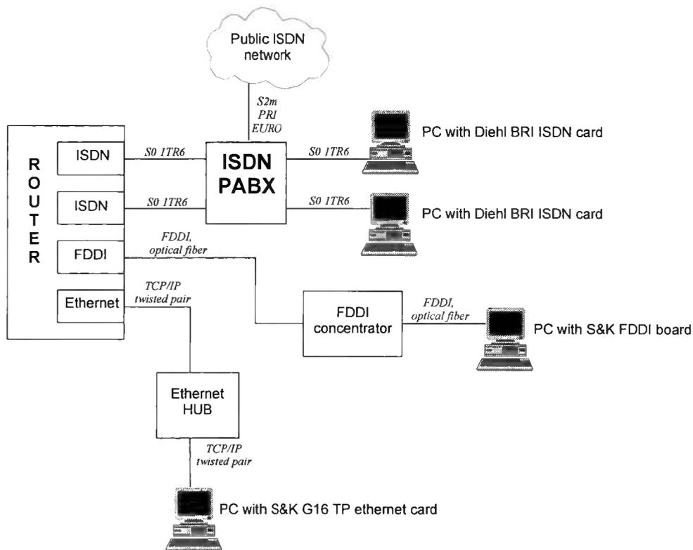
**Figure 5.5** ISDN remote dial-in configuration
